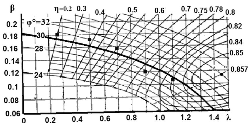
Fig.2.2. Dependences of  $\beta$  ( $\lambda$ ) and  $\eta$  ( $\lambda$ ) at installation angle  $\varphi = 30^\circ$  for three-bladed screw (points- calculation, line - experiment).
