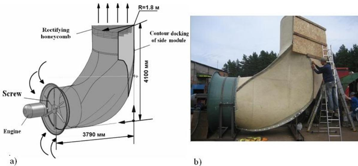
Fig. 2.8. Natural module of wind tunnel with a fan and motor, a) Computer model, b) Natural tunnel
