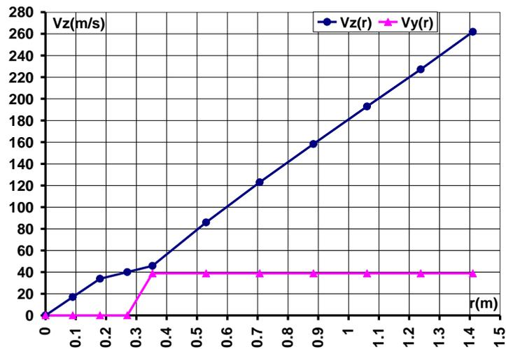
Fig. 2.9. Character of the changes of vertical velocity  $V_y$  (-▲-) and the linear rotation velocity  $V_z$  (-●-) of the flow along the radius of the airscrew.
