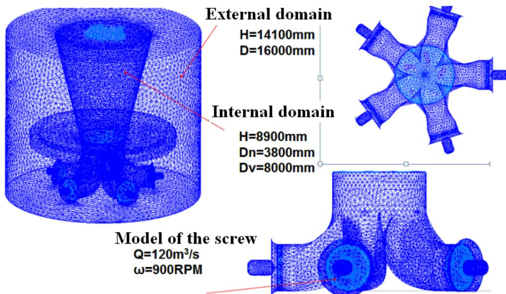
Fig. 3.6. Finite element computational model of optimized tunnel with natural dimensions
