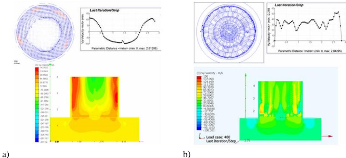
Fig.3.3. a) Distribution pattern of flow swirling and vertical velocity component ( $V_y$ ) in absence of air flow rectifying device. b) Distribution pattern of flow swirling and vertical velocity component ( $V_y$ ) of air flow after installation of the rectifying device.
