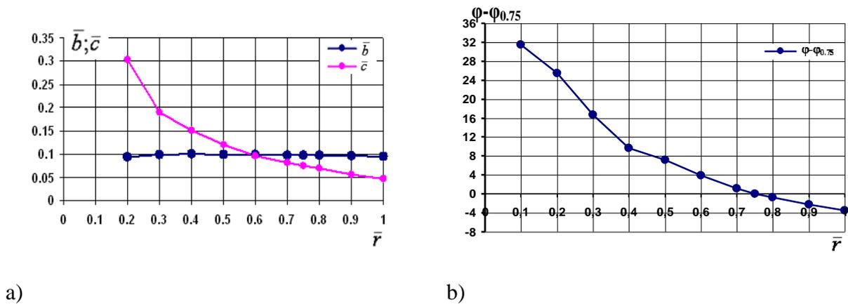
Fig. 2.3. Geometrical characteristics of the blade of refurbished screw. a) Relative chord and relative thickness; b) Twist of blade.
