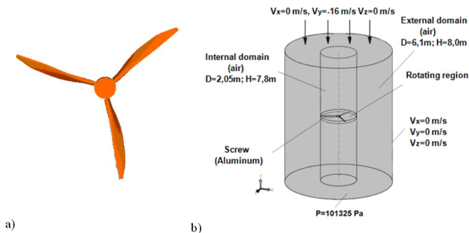
Fig. 2.1. Models of three-bladed screw: a) Geometric computer model of screw; b) Computational model of screw model in a wind tunnel.
