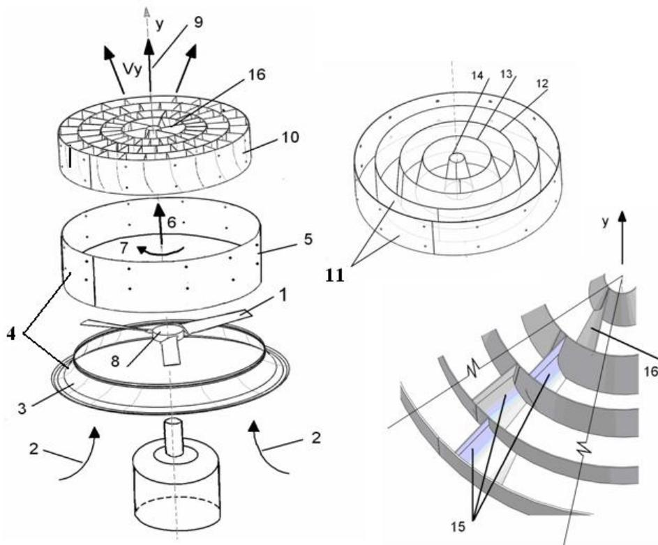
Fig.3.1. Construction elements of generator of vertical air jet
