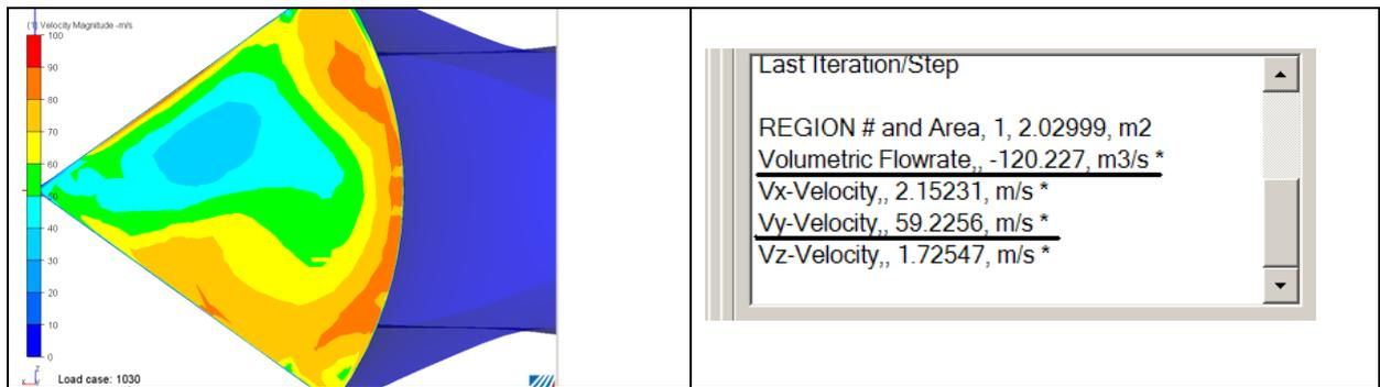
Figure 2.10. a) Picture of distribution of velocity  $V_y(r)$  in the outlet section of computer model of the experimental device; b) The results of calculation in the program CFdesign of the parameters averaged in cross-section.
