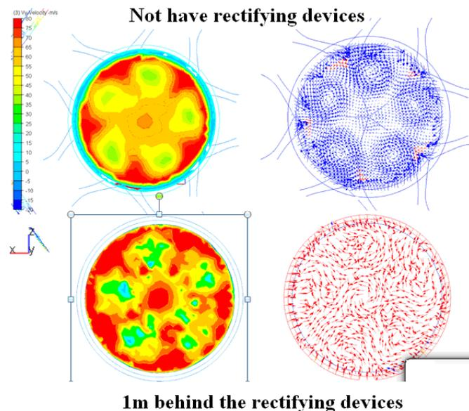
Fig.3.7. Distribution pattern of vertical velocity and swirling zones in the jet.
