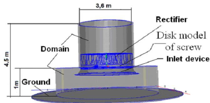
Fig.3.2. The computational diagram of the generator of air jet with the domain
