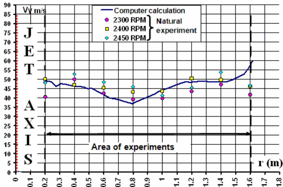
Figure 2.11. Comparison of results of numerical calculations and experiments of determination of vertical velocity  $V_y(r)$  in jet in the exit of the module of the experimental device.
