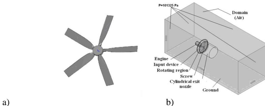
Fig. 2.4. a) Geometrical model of five - blade screw; b) Screw in a short channel with inlet device and cylindrical exit nozzle.
