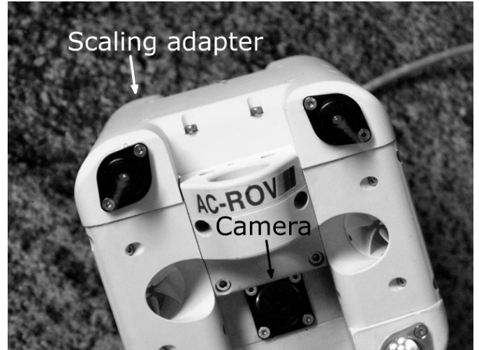
Fig. 12. Laser scaling adapter installed on ROV – front view (3)
