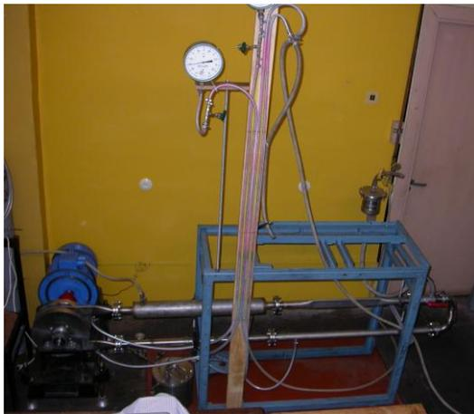
Fig.3.2. Experimental InGaSn circuit for testing electromagnetic induction pump with rotating PM
