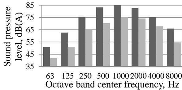
4.20. fig. Measured (dark) and CadnaA calculated (light) spectrums of electric train pass by noise
