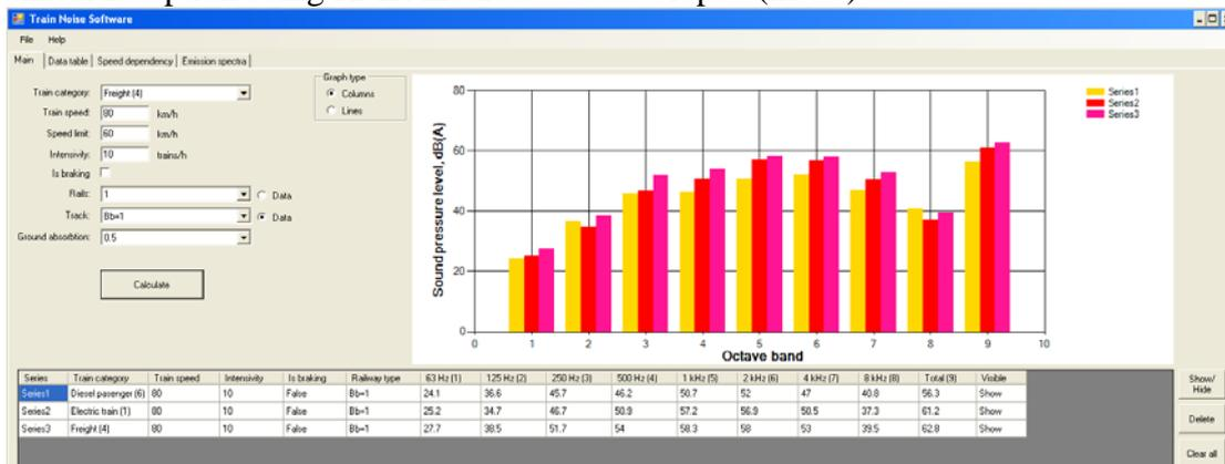
4.25. fig. TNS GUI - pass by noise spectra calculation
