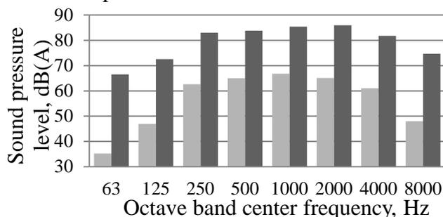
4.22. fig. Measured (dark) and CadnaA calculated (light) spectrums of mixed freight train pass by noise
