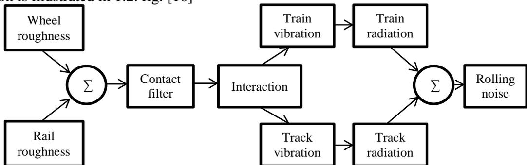
1.2. fig. The mechanism of rolling noise generation
