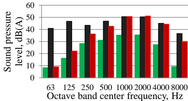
5.7. fig. CadnaA calculated and measured spectrums
