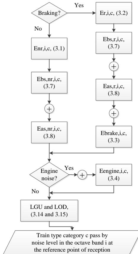
4.26. fig. TNS calculation algorithm
