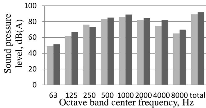
4.4. fig. Pass by noise level of electric train, dark-grinded, light - non-grinded track
