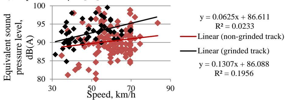
4.7. fig. Freight train pass by noise level speed dependency
