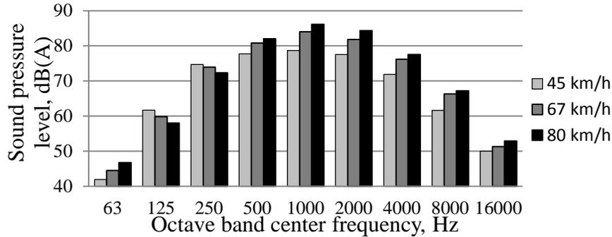
4.11. fig. Pass by noise spectrums of electric trains at different speeds
