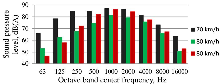
4.14. fig. Pass by noise spectrums of different trains
