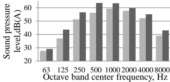
4.23. fig. Pass by noise spectrums, track with joints (dark) and jointless track (light) electric train, train speed 60 km/h, pass by time 7.2 s
