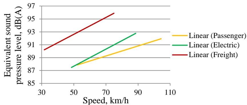
4.9. fig. Pass by noise level speed dependency of trains on grinded track
