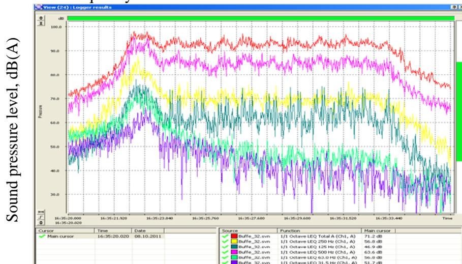
4.16. fig. Pass by noise levels of diesel passenger train in the time and frequency domain
