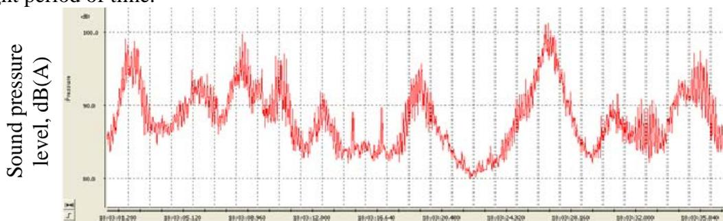
4.15. fig. Freight mixed train pass by noise level, dB(A) in the time domain
