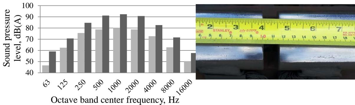
4.18. fig. Electric train pass by noise spectrums, dark – rails with joint; light – jointless rails
