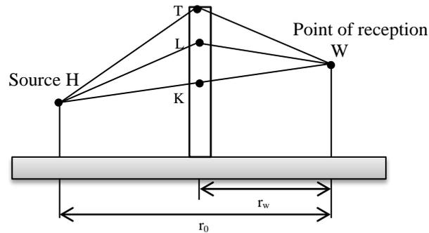
3.2. fig. The idealized barrier between source and point of signal reception
