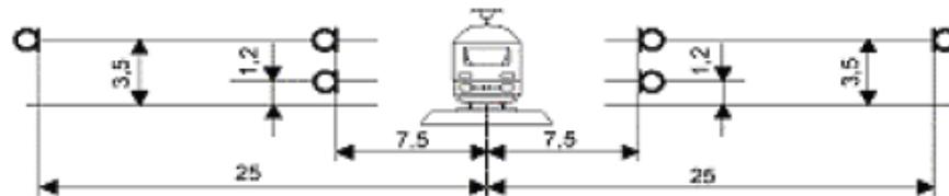
4.1. fig. Microphone position at the test site, distances and heights are in meters
