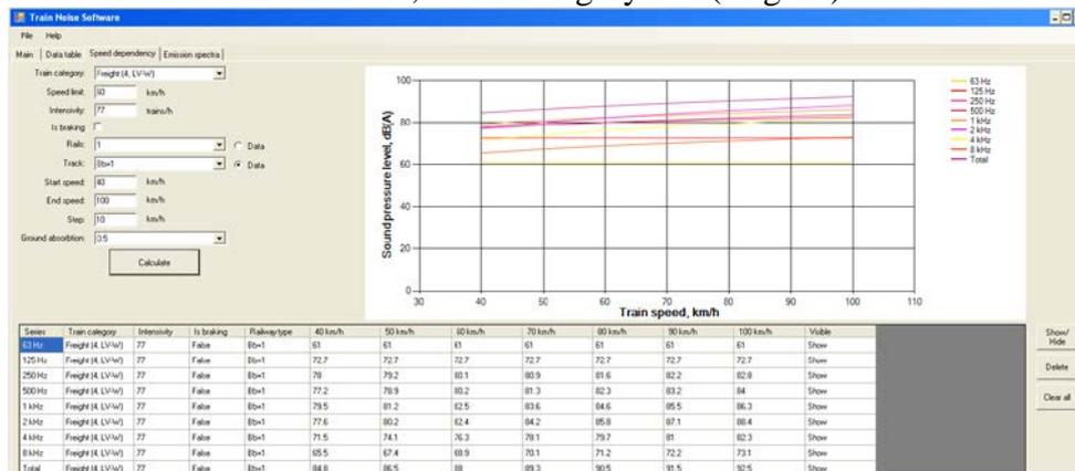
4.30. fig. Pass by noise level speed dependency of Latvian freight trains consisting only from wagons, calculated using TNS
