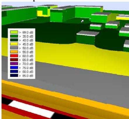
5.2. fig. CadnaA noise map of Plavinas gymnasium area in 3D view calculated using RMR method and traffic intensity data
