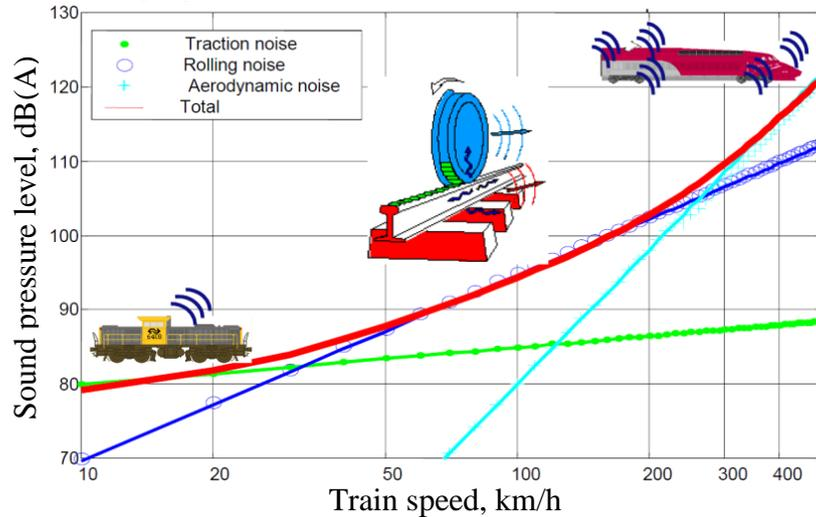
1.1. fig. Railway noise sources and typical dependency on train speed
