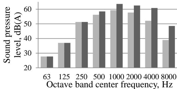
4.24. fig. CadnaA calculated pass by noise spectrums for braking (dark) and non-braking (light) electric train train speed 60 km/h, pass by time 7.2 s
