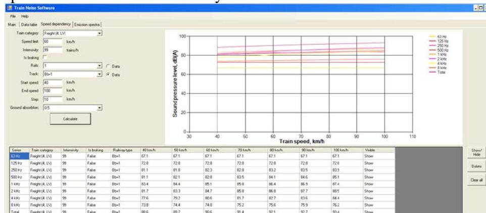
4.29. fig. TNS calculated Latvian mixed freight train pass by noise level speed dependency
