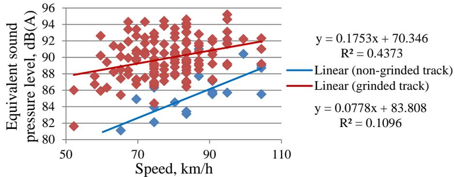
4.6. fig. Diesel passenger train pass by noise level speed dependency
