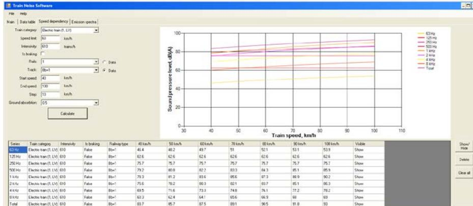
4.27. fig. TNS calculated Latvian electric train pass by noise level speed dependency
