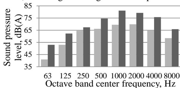
4.19. fig. Measured (dark) and CadnaA calculated (light) spectrums of diesel passenger train pass by noise
