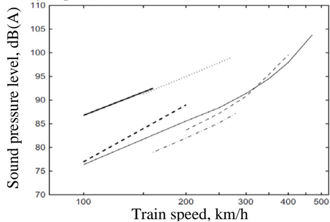
1.3. fig. Measurement results of train pass-by noise from different types of trains
