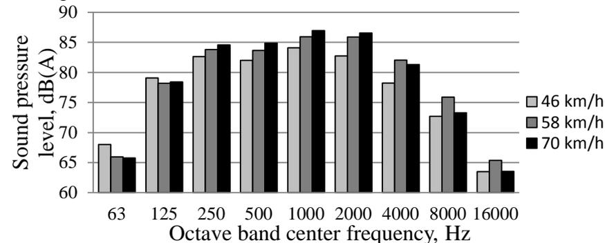
4.13. fig. Pass by noise spectrums of freight mixed trains at different speeds
