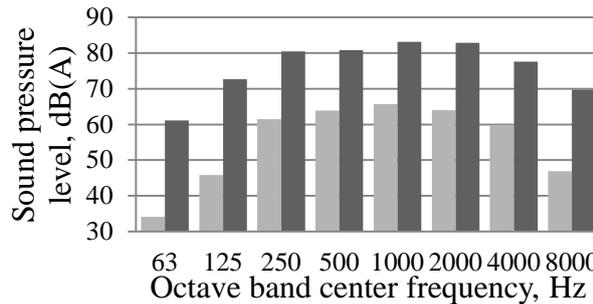
4.21. fig. Measured (dark) and CadnaA calculated (light) pass by noise spectrums of freight train consisting only from wagons
