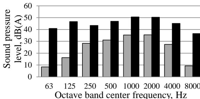
5.3. fig. CadnaA calculated (light) and measured (dark) noise spectrums at the reference point of reception near Plavinas gymnasium
