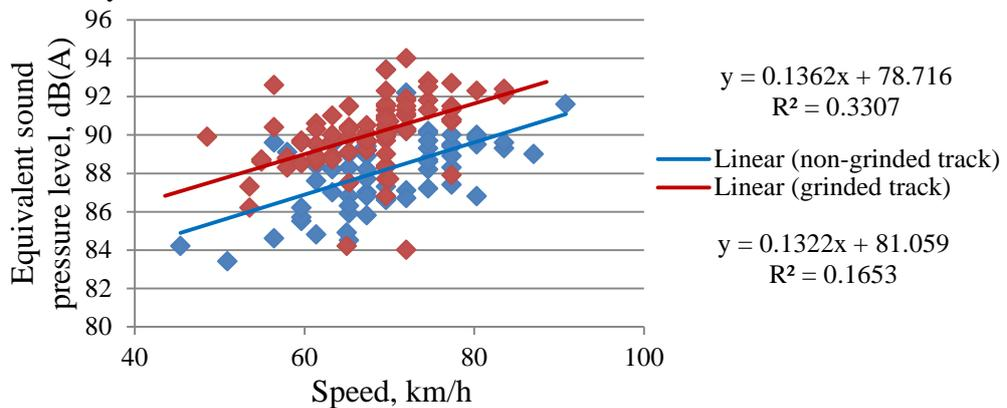
4.5. fig. Electric train pass by noise level speed dependency
