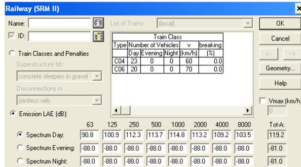
5.6. fig. TNS calculated radiation spectrum used as input data for CadnaA calculations
