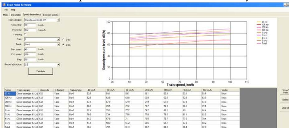
4.28. fig. TNS calculated Latvian diesel train pass by noise level speed dependency
