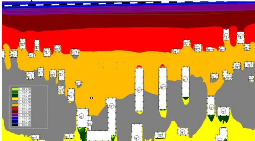
5.4. fig. CadnaA noise map of Plavinas gymnasium area in 2D view calculated using RMR and updated based on measurement results
