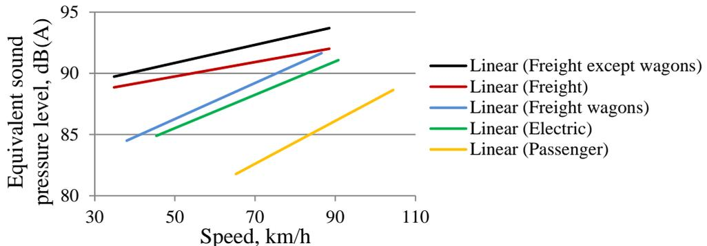
4.10. fig. Pass by noise level speed dependency of trains on non-grinded track
