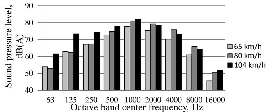
4.12. fig. Pass by noise spectrums of diesel passenger trains at different speeds
