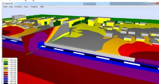
6.2. fig. CadnaA modeled noise reduction by 4 m high and 200 m long noise barrier
