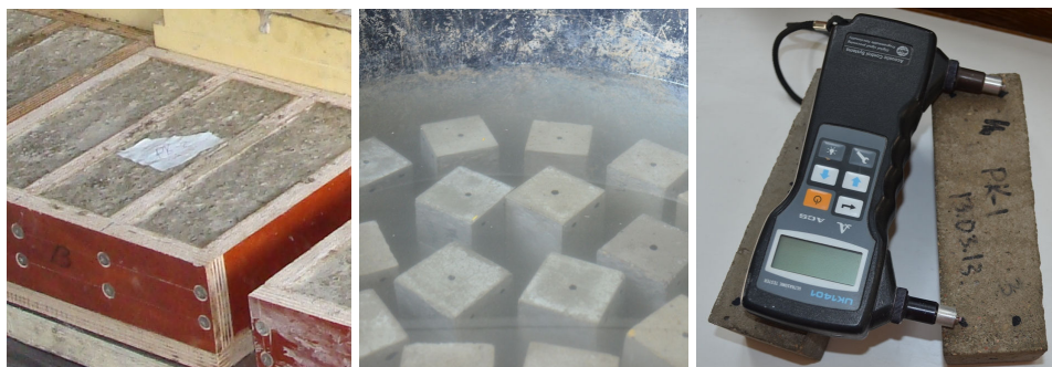
Figure 4 – Produced prismatic shape concrete specimens for frost resistance test
