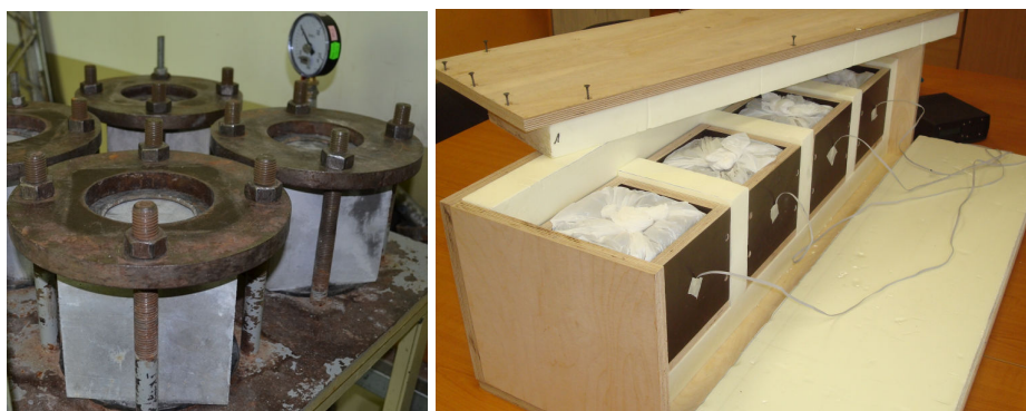
Figure 3 – Equipment to measure permeability (left) and hydration temperature inside of concrete mixtures (right).
