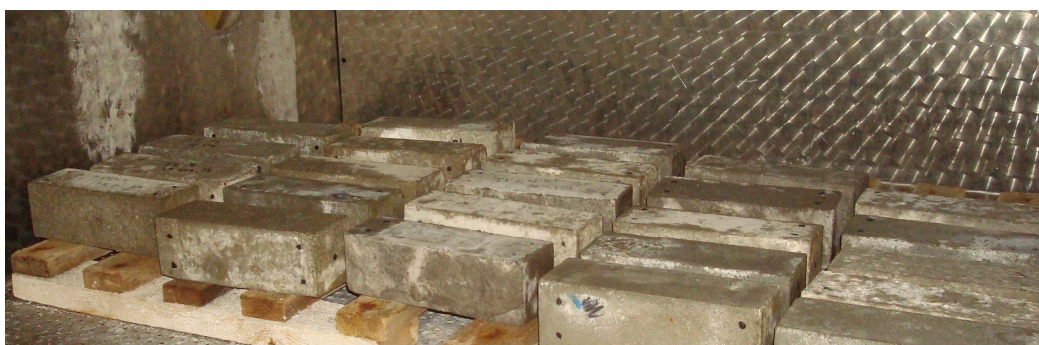
Figure 5 - Concrete specimens in the climatic chamber ILKA KTK-800
