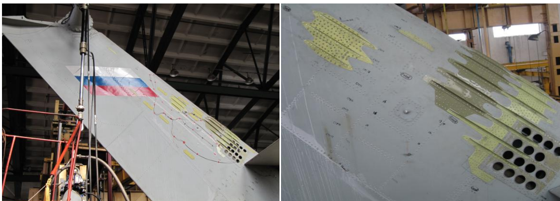
Fig.5.11 The general view of repaired cracks on keel beam of helicopter Mil-26
