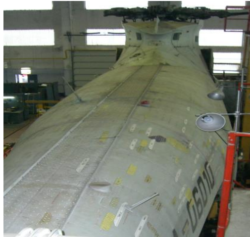
Fig.5.7 The general view of tail beam's cracking after fatigue test loading.
