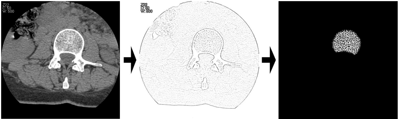
Fig. 6. Extracting the cortical bone from inside the contour, input medical image (left), inverse Laplace filter applied to the medical image (in the middle).
