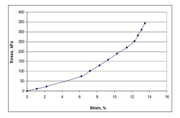
Fig.3. Dependence of strain and stress for vascular implant reinforced of natural silk yarns
