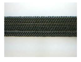
Fig.2. Prototype of innovative woven vascular implant
