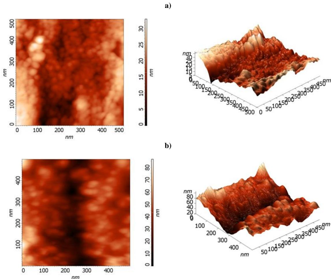
9. Fig. The topographic pictures of the cotton textile treated by sol
