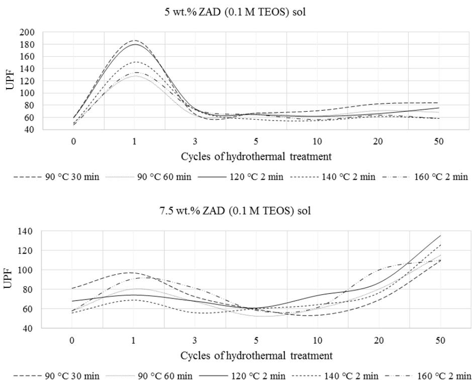
17. Fig. UPF values of the modified textiles after hydrothermal treatment
