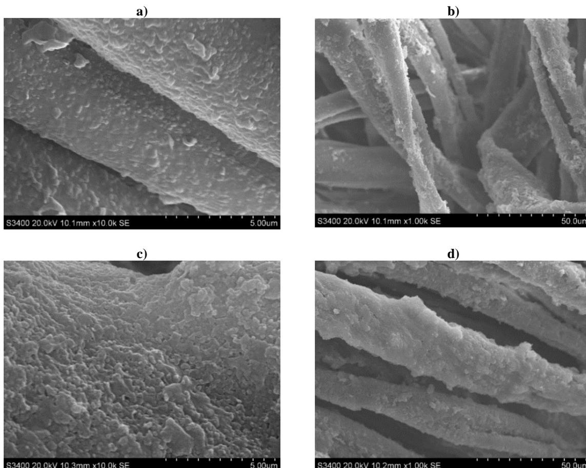
Fig. 6 The coating structure of the cotton textile modified by 7.5 wt. % ZAD (0.1 M TEOS) sol (thermal post-treatment 120 °C at temperature 2 min)
