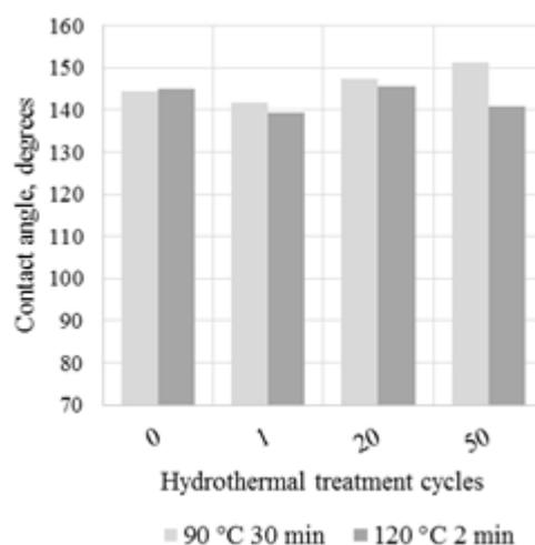
Fig. 19 Contact angle of the cotton textiles modified by 7.5 wt. % ZAD (0.1 M TEOS) sol
