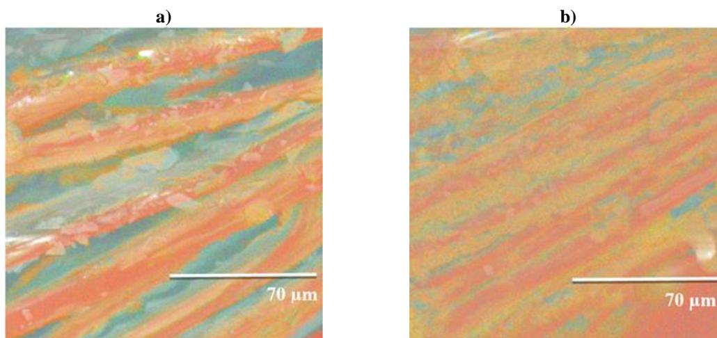
Fig. 7 The distribution of the chemical elements F, Si, Zn in the coating of the modified cotton textile surface (thermal post-treatment at 120 °C temperature 2 min.)
