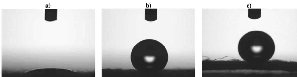
Fig. 18 Cotton textile surface wettability process (drop 5µL)
