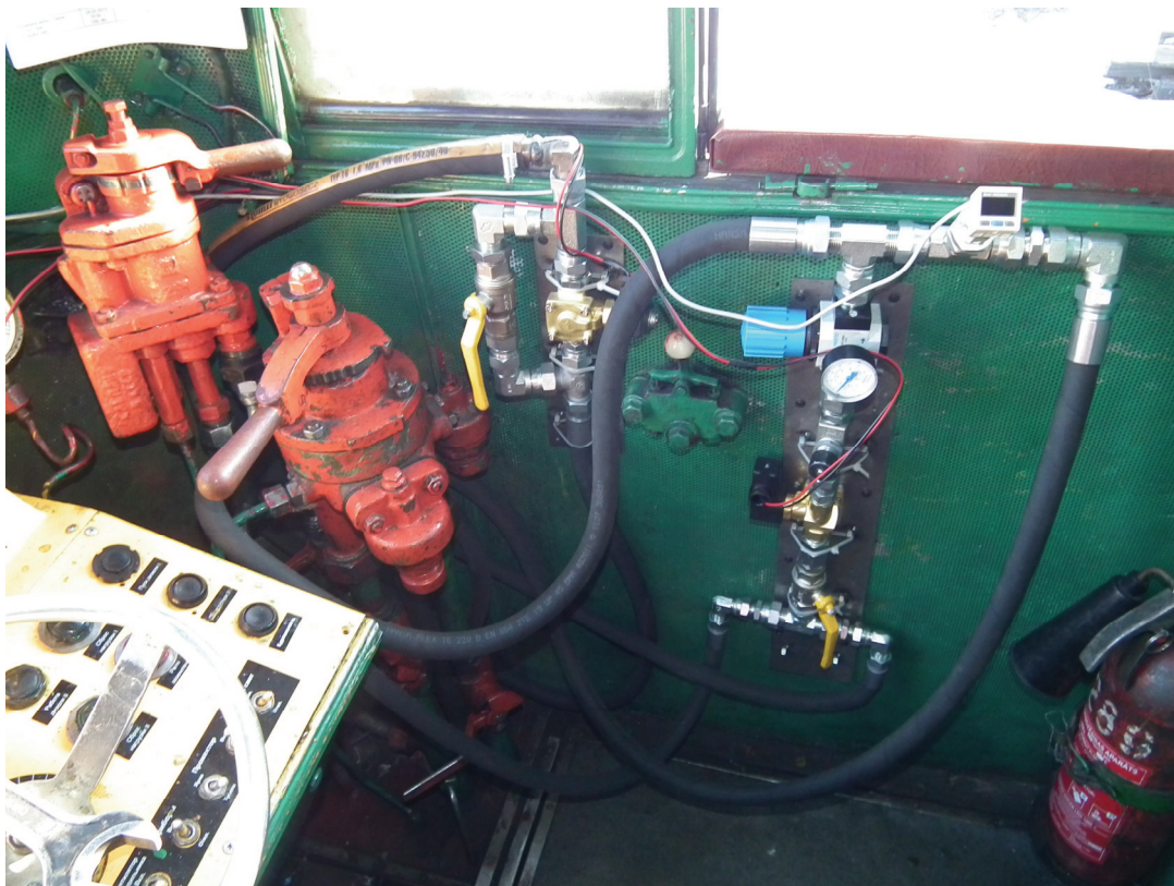
Fig. 17. Pneumatic part of the SAFE-R 5 prototype device connection to the locomotive M62
