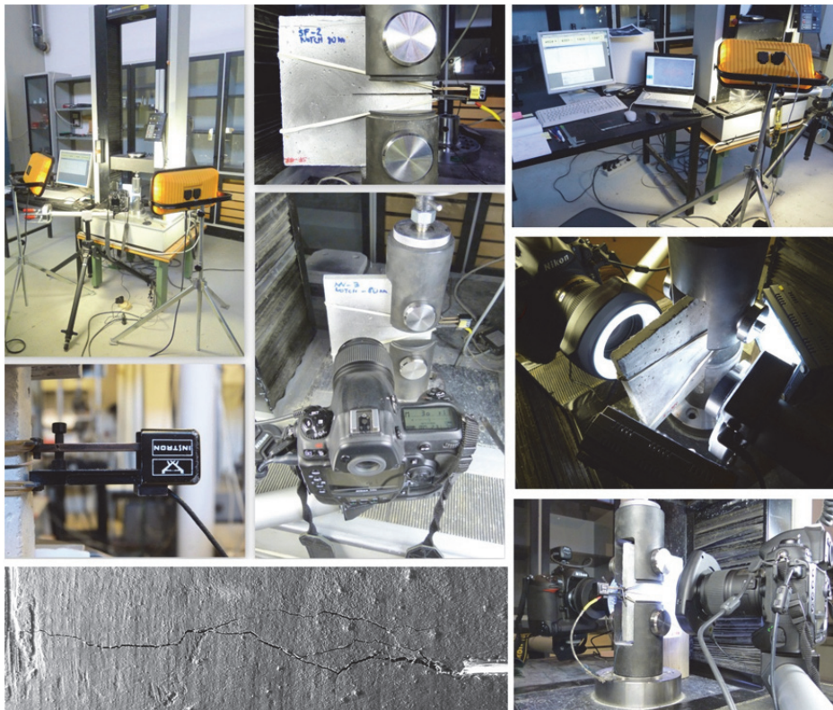
Fig. 3.3. Determination of tensile strength and uniaxial tensile crack development research (DTU lab)
