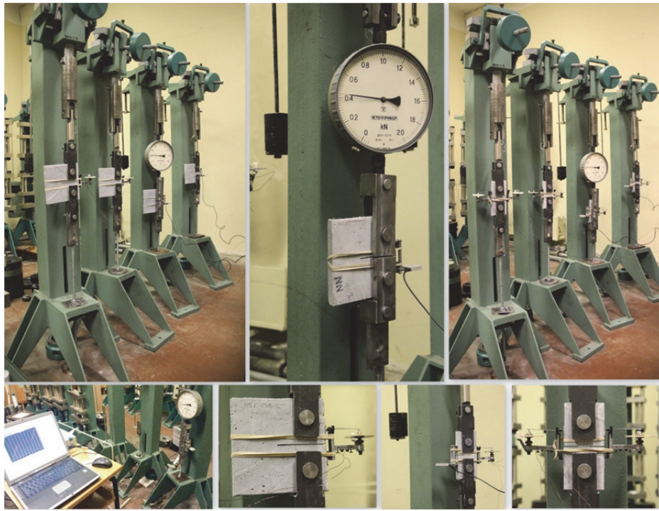
Fig. 3.2. Determination of uniaxial tensile creep strains (RTU lab)
