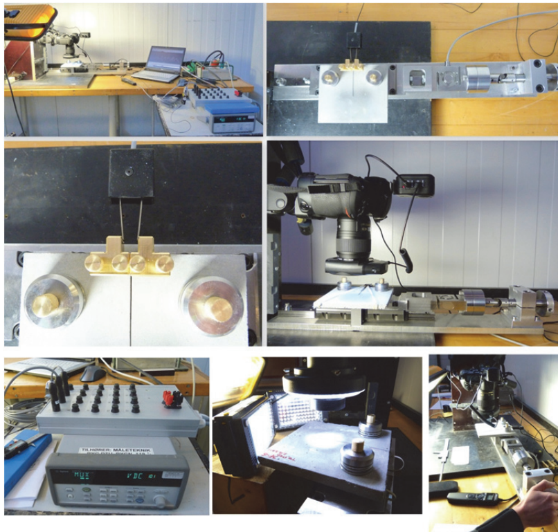
Fig. 3.4. Determination of tensile strength and uniaxial tensile crack development research with the new DTU tensile test stand (DTU lab)
