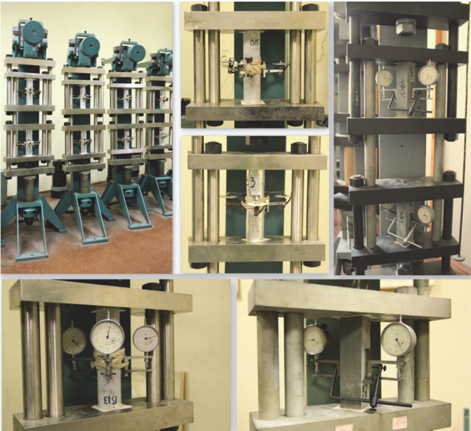
Fig. 3.1. Determination of uniaxial compression creep strains (RTU lab)
