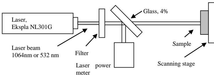
Figure 3.1. The schematic of the laser irradiation setup.
