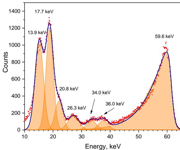
Figure 4.11 Best fit results for  $^{241}\text{Am}$   $\gamma$ -ray spectrum of laser irradiated CdZnTe detector crystal
