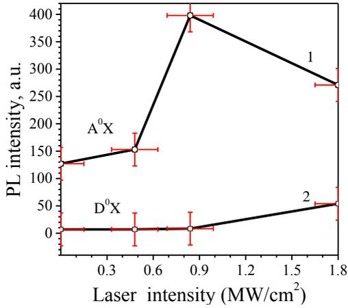
Figure 4.3 The PL intensity of A<sup>0</sup>X (1) and D<sup>0</sup>X (2) bands of CdZnTe crystal as a function of Nd:YAG laser intensity: irradiated by the laser.
