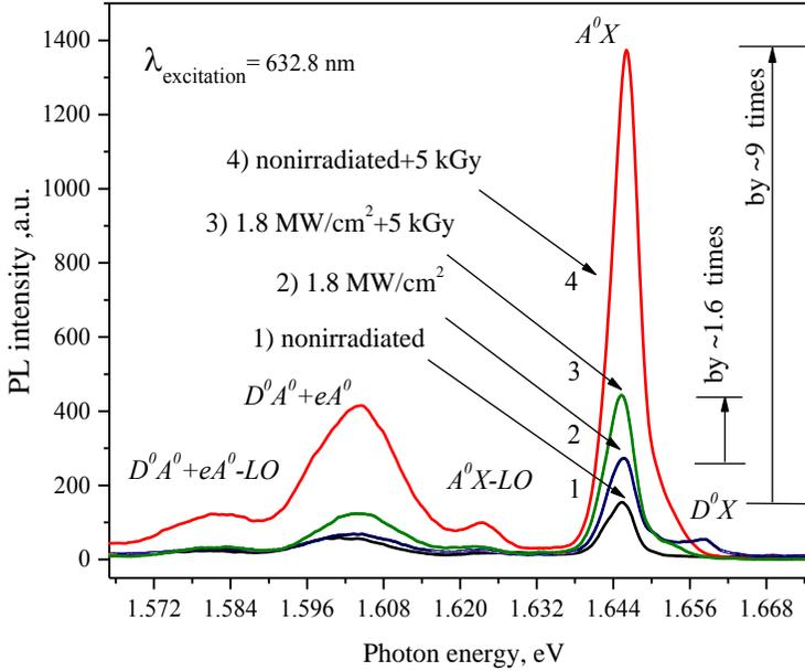
Figure 4.2 The PL spectra of  $\text{Cd}_{0.9}\text{Zn}_{0.1}\text{Te}$  crystal before 1 and after irradiation by Nd:YAG laser: 2 - irradiated by Nd:YAG laser with intensity  $1.8 \text{ MW/cm}^2$ ; 3 – previously irradiated by Nd:YAG laser with intensity  $1.8 \text{ MW/cm}^2$  and subsequently by  $\gamma$ -ray with a dose rate of  $5.0 \text{ kGy}$ ; 4 – irradiated by  $\gamma$ -ray with a dose rate of  $5.0 \text{ kGy}$ .
