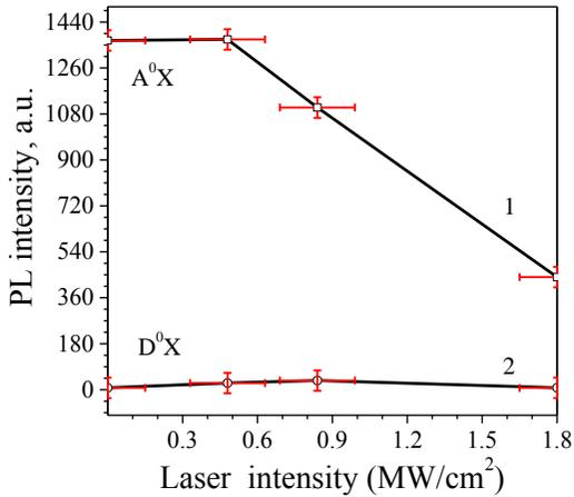
Figure 4.4 The PL intensity of A<sup>0</sup>X (1) and D<sup>0</sup>X (2) bands of CdZnTe crystal as a function of Nd:YAG laser intensity: irradiated by the laser and after subsequently irradiation by  $\gamma$ -ray with a dose rate of 5.0 kGy.
