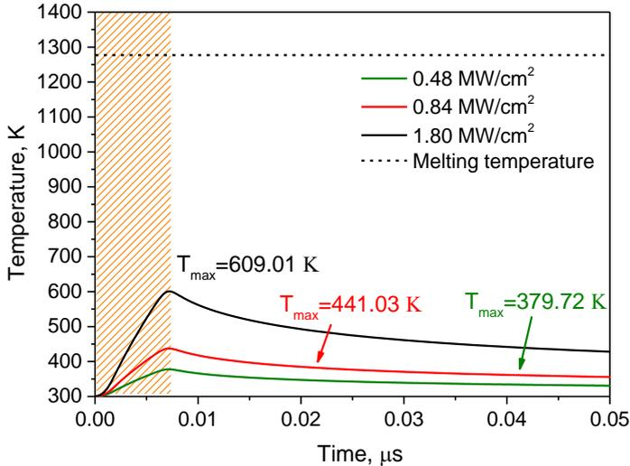
Figure 4.1 The calculated time dependence of the temperature of the laser irradiated CdZnTe sample by different laser intensities. Striped area represents the laser pulse duration.
