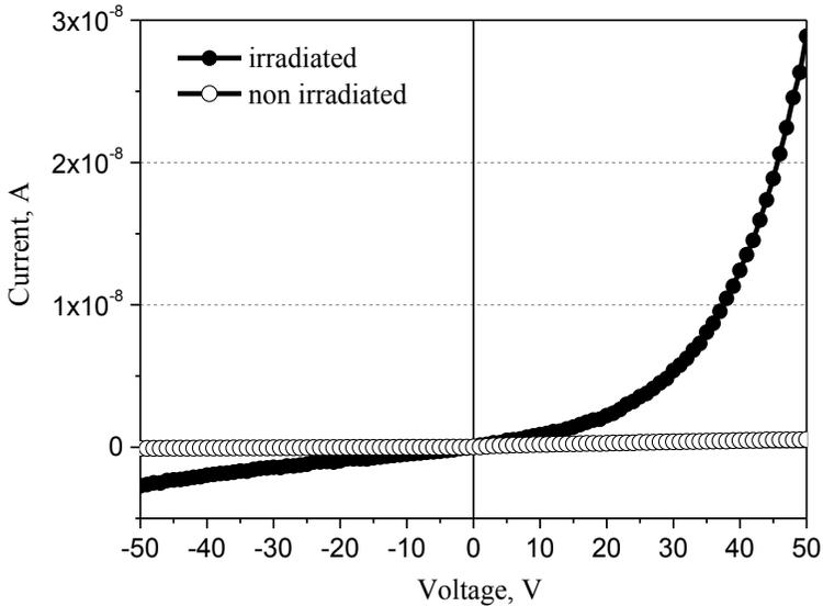
Figure 4.6. I-V characteristics of CdTe/CdZnTe heterojunction
