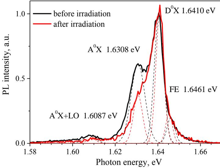
Figure 4.9 PL spectra of CdZnTe samples before (curve 1) and after irradiation (curve 2 -with pulse number  $3.6 \times 10^4$  pulses) by the Nd:YAG laser.
