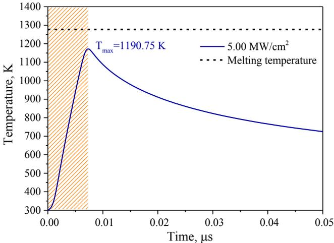
Figure 4.5 The calculated time dependence of the temperature of the laser irradiated CdZnTe sample by different laser intensities. Striped area represents the laser pulse duration.
