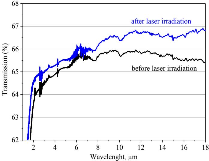
Figure 4.8. FTIR spectra of CdZnTe samples before (curve 2) and after irradiation (curve 1) by the Nd:YAG laser.
