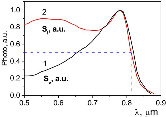
Figure 4.7 Photosensitivity spectra in contacts on the non-irradiated (1) and irradiated (2) surfaces measured in the short-circuit current mode at  $T = 295$  K.
