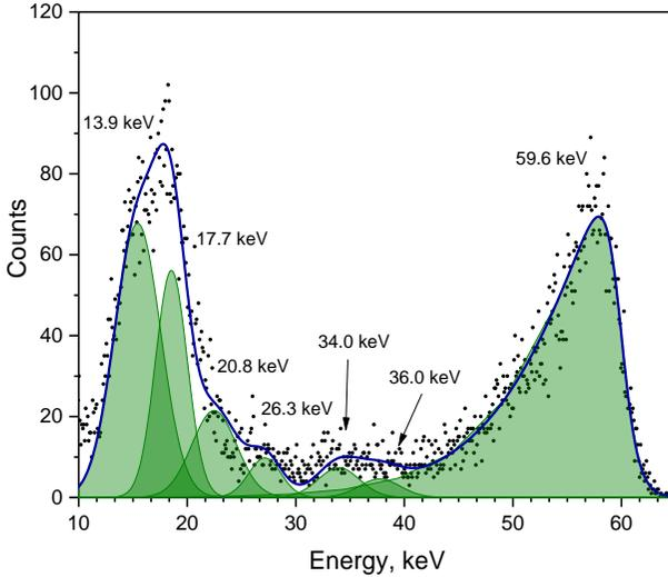
Figure 4.10 Best fit results for  $^{241}\text{Am}$   $\gamma$ -ray spectrum CdZnTe detector crystal before laser irradiation.
