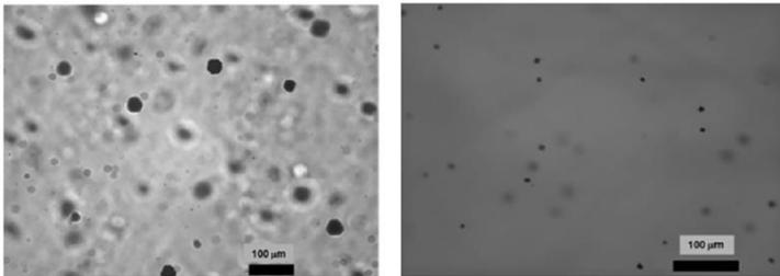
Figure 2.1 IR microscopy images of Te inclusions inside the CdZnTe crystal [20].
