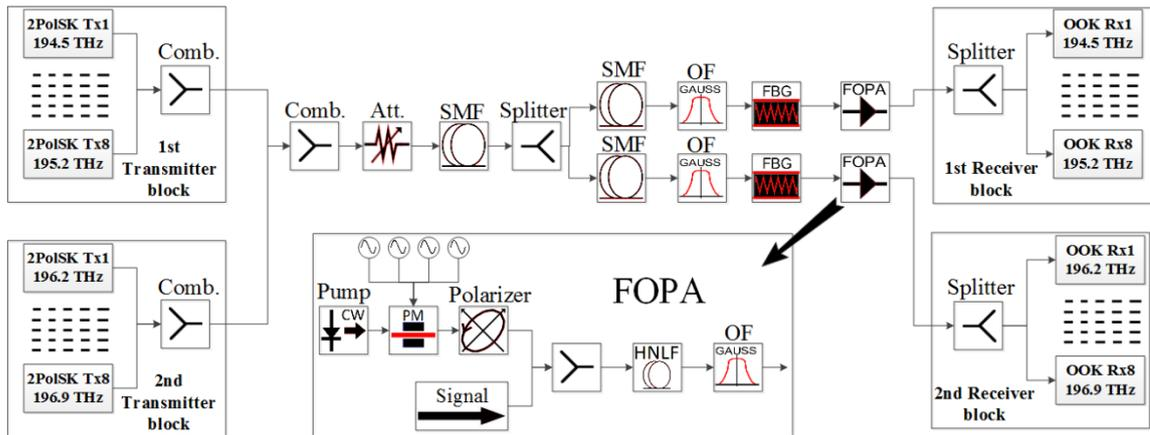
Fig. 18. Simulation model of the 16-channel WDM transmission system with two access network branches, where in each branch the FOPA pre-amplifier is used for 2PolSK to NRZ-OOK modulation format conversion.
