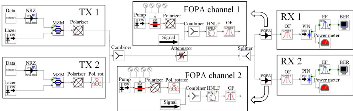
*Fig. 21.* Simulation model of the two-channel optical transmission system with FOPA for division and amplification of polarisation multiplexed signals.
