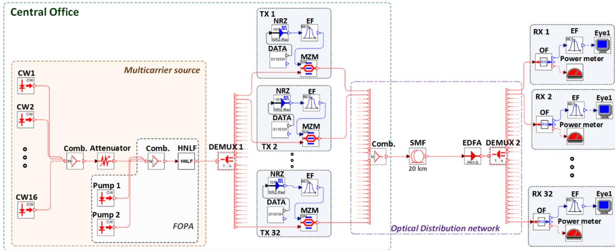
Fig. 12. Simulation model of the 32 channel 10 Gbps WDM transmission system with the provided multicarrier source solution, which is based on wavelength conversion using a dual-pump FOPA.
