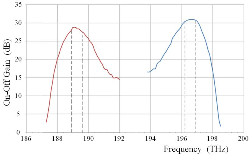
Fig. 19. Gain spectrum ensured by the FOPA with 790 mW 1554.15 nm linearly polarised pumping radiation at initial signal frequencies (blue line) and idler frequencies (red line).
