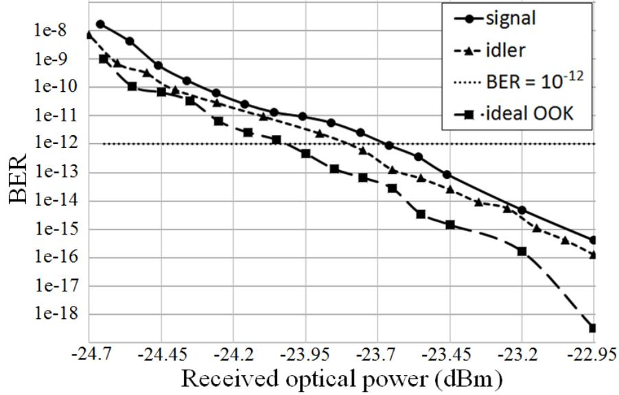
Fig. 17. BER value dependence on the detected signal power in the standard single-channel transmission system (dashed line), and in the system with modulation format conversion at the initial signal frequency (solid line) and at idler frequency (dotted line).
