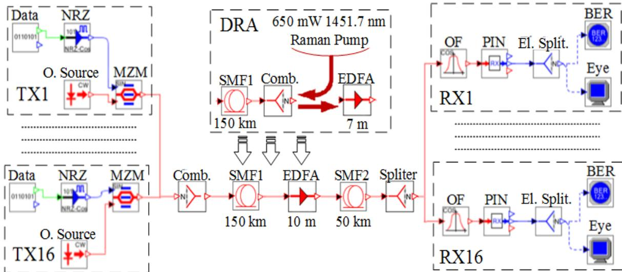
Fig. 4. Simulation model of the 16-channel 10 Gbps DWDM transmission system with an EDFA inline amplifier or with a hybrid Raman-EDFA amplifier.
