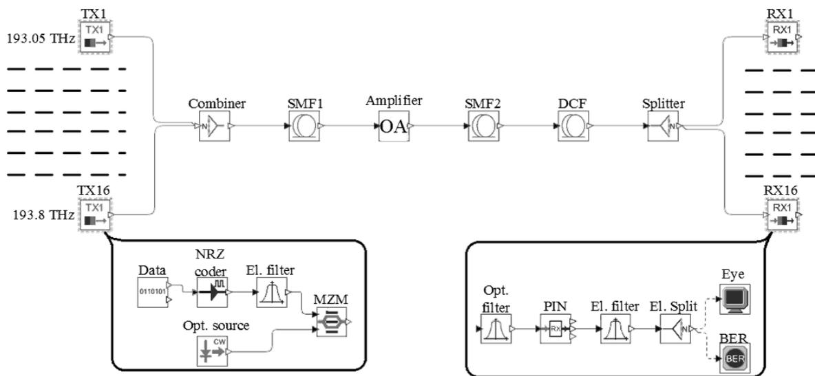
Fig.2. Simulation model of the 16-channel 10 Gbps DWDM transmission system used for comparison of optical amplifier performance.
