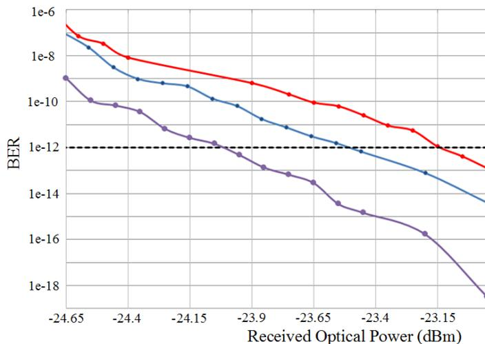
Fig. 20. BER value dependence on the detected signal power in the standard 8-channel transmission system (violet), and in the 5<sup>th</sup> channel on the 2<sup>nd</sup> branch of the multi-channel system with modulation format conversion at the initial signal frequency (blue) and idler frequency (red).
