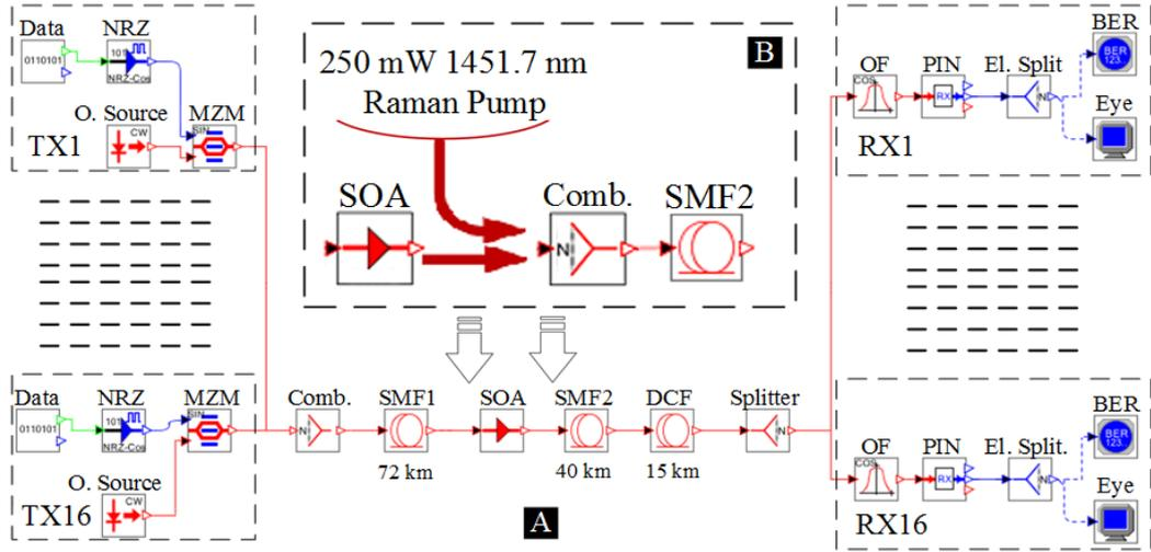
Fig. 7. Simulation model of the 16-channel 10 Gbps DWDM transmission system with the SOA inline amplifier (a) or with a hybrid Raman-SOA amplifier (b).
