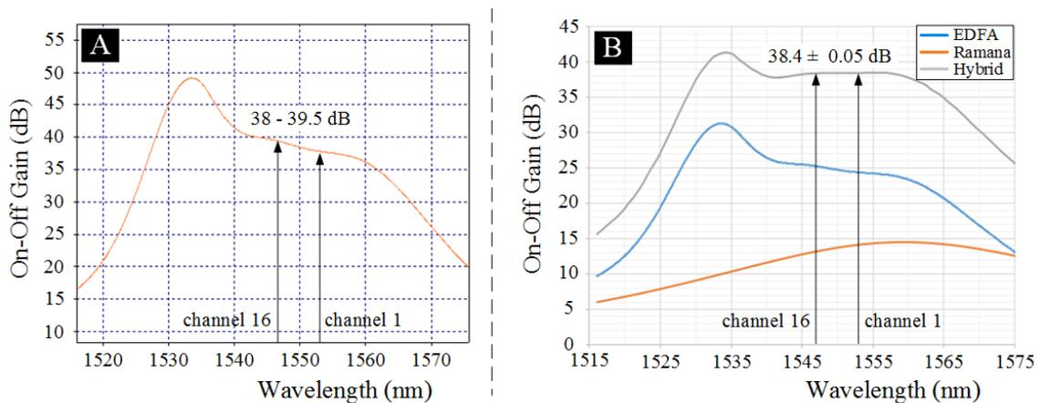
Fig. 5. Gain spectra of the EDFA inline amplifier (A) and of the hybrid Raman-EDFA amplifier (B).
