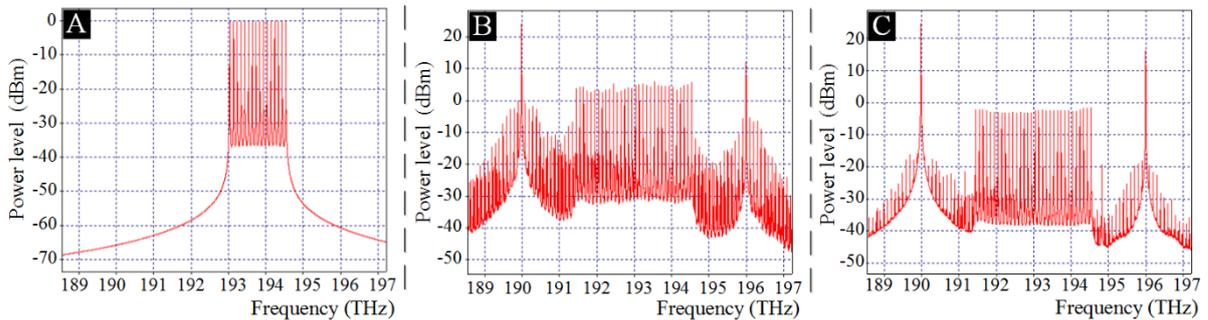
Fig. 13. Optical spectrum at the input of the FOPA when initial carrier power is set to 0 dBm (a), and optical spectra at the output of the HNLFF when the power of the initial carriers is set to 0 dBm (b) and to -10 dBm (c).
