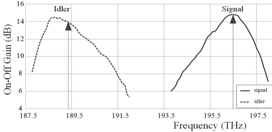
Fig. 16. Gain spectrum produced by the single-pump FOPA with linearly polarised pumping radiation at signal frequencies (solid line) and at idler frequencies (dotted line).
