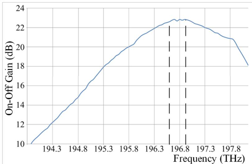
Fig. 9. Gain spectrum of the single-pump FOPA with 660 mW 1553.9 nm pumping radiation.
