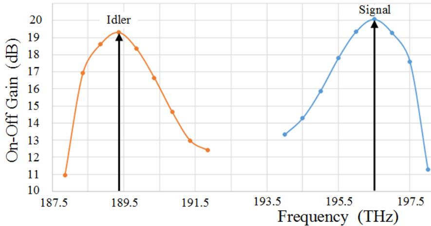
Fig. 22. FOPA produced on-off gain for the 1<sup>st</sup> channel at idler frequencies (orange line) and at the initial signal frequencies (blue line).
