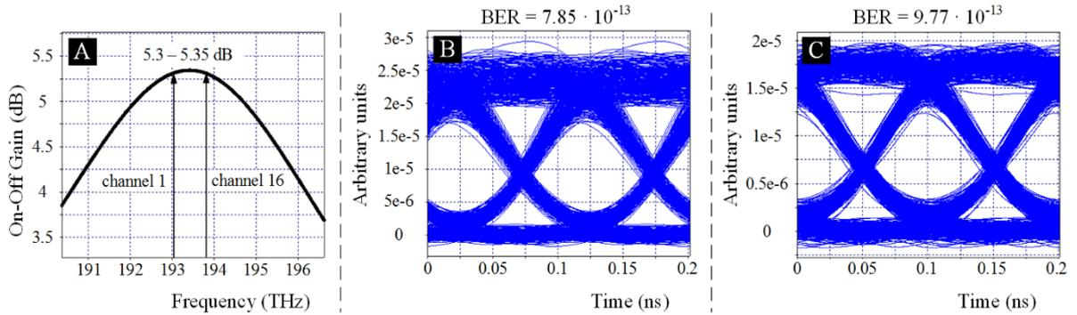
Fig. 8. DRA produced gain spectrum (a) and eye diagrams of the 9<sup>th</sup> channel in the system with the SOA inline amplifier (b) and the 10<sup>th</sup> channel in the system with the Raman-SOA hybrid amplifier (c).
