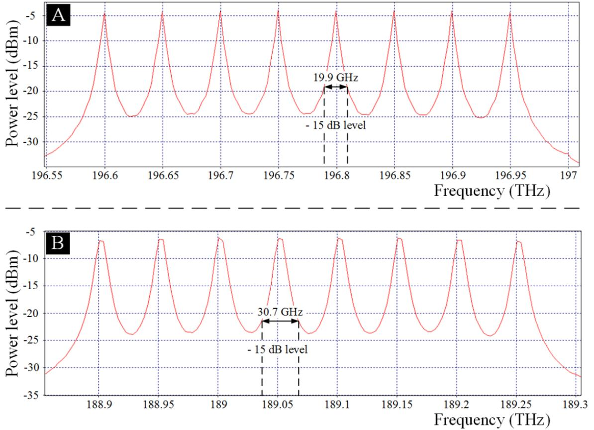
Fig. 10. Spectra of the amplified signal (A) and the generated idlers (B) at the output of the single-pump FOPA.
