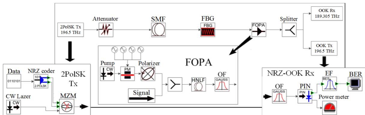
*Fig. 15.* Simulation model of the single-channel transmission system, where a single-pump FOPA with linearly polarised pumping radiation is used for 2PolSK to NRZ-OOK modulation format conversion.
