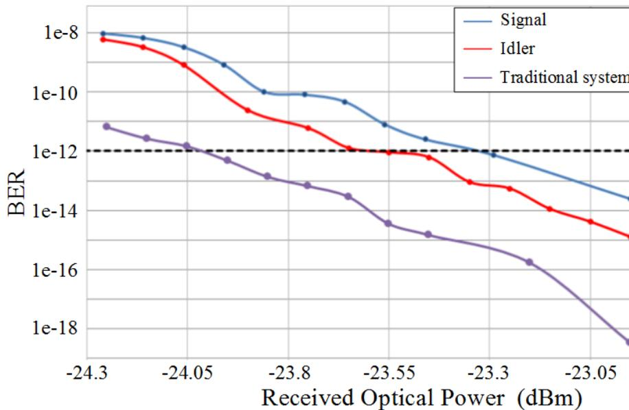
Fig.23. BER value dependence on the power of the detected signal in the standard single-channel system (violet) and in the 1<sup>st</sup> channel of the system with the chosen FOPA configuration of the signal at its initial frequency (blue) and of the idler (red).
