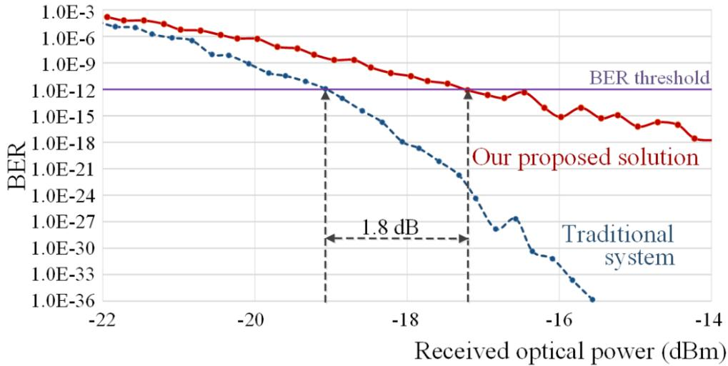
Fig. 14. BER value dependence on the power of the detected signal for the 12<sup>th</sup> channel in the system with the proposed multicarrier source solution (red line) and in the system with traditional architecture (blue line).
