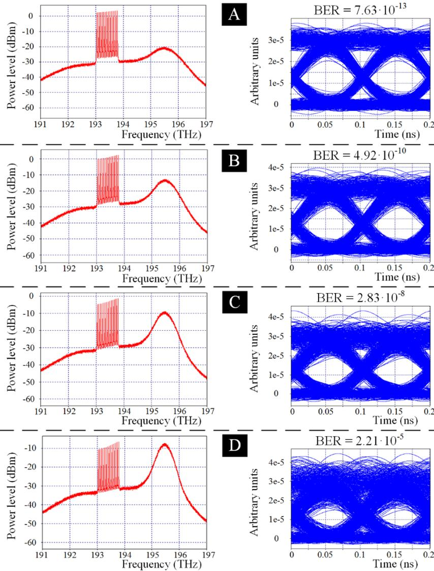
Fig. 3. Optical spectra at the output of the EDFAs (to the left) and Eye diagrams of the signal detected in the 9<sup>th</sup> channel (to the right) after 1<sup>st</sup> (a), 2<sup>nd</sup> (b), 3<sup>rd</sup> (c) and 4<sup>th</sup> (d) stages of amplification.
