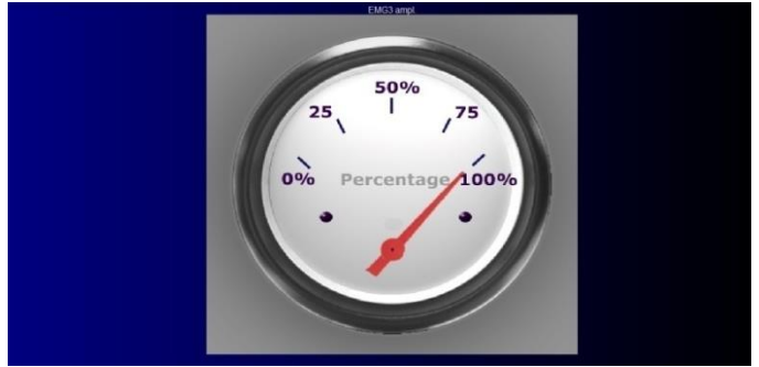
Fig. 7. Visualisation “speedometer” – when the muscle biopotential is above the selected level, speedometer reading increases. If the muscle biopotential decreases under the threshold, the reading decreases.
