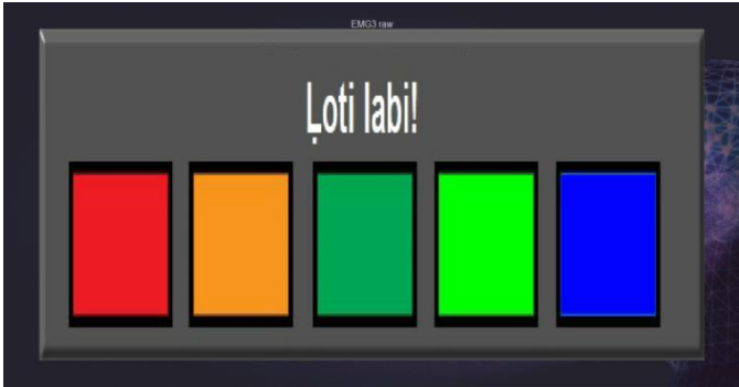
Fig. 11. Visualisation “power level” – If the muscle biopotential is below the threshold, there are no colours displayed. When the biopotential reaches the threshold level, the red colour is displayed. If the muscle biopotential is held above the threshold, orange, green and blue colours are displayed consecutively.
