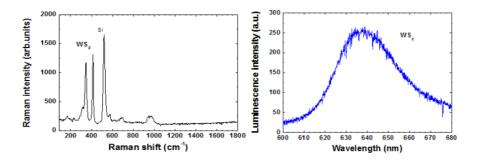
Figure 7: Measured Raman (*left*) and luminescence (*right*) spectrum of a WS<sub>2</sub> nanostructure on a silica wafer.
