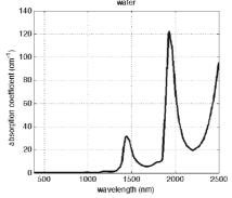
Figure 12: The absorption coefficient of water in  $cm^{-1}$  (380-2500nm), with a resolution of 5 nm [2]
