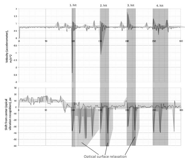
FIGURE 1 Verification of optical vibration recognition with using piezo accelerometer
