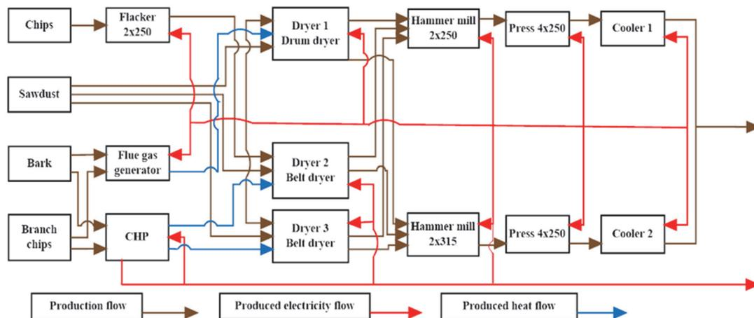
Fig. 2.1. Operational scheme of a pellet production unit.
