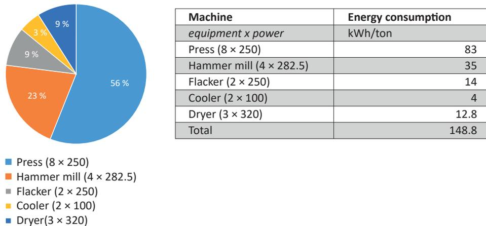
Fig. 1.1. Electricity consumption of an equipment per ton of production.
