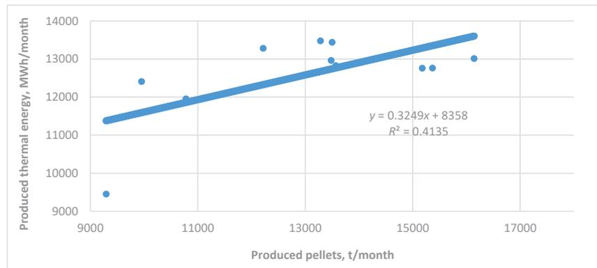
Fig. 1.3. Volume of production depending on the heat generated in a cogeneration plant.
