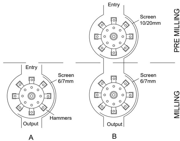
Fig. 2.2. Principal scheme of a hammer mill.
