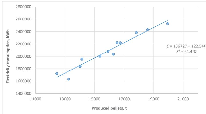
Fig. 1.2. Electricity consumption of an equipment per produced volume of pellets.
