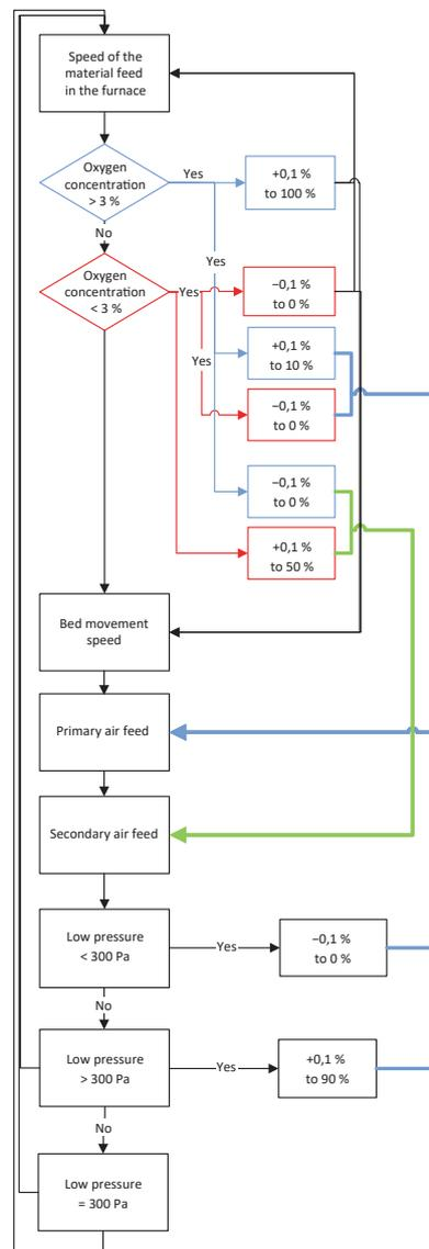
Fig. 3.1. Algorithm of the automatic control system.
