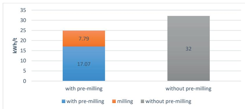
Fig. 2.3. Milling regime of electricity consumption, kWh/t.
