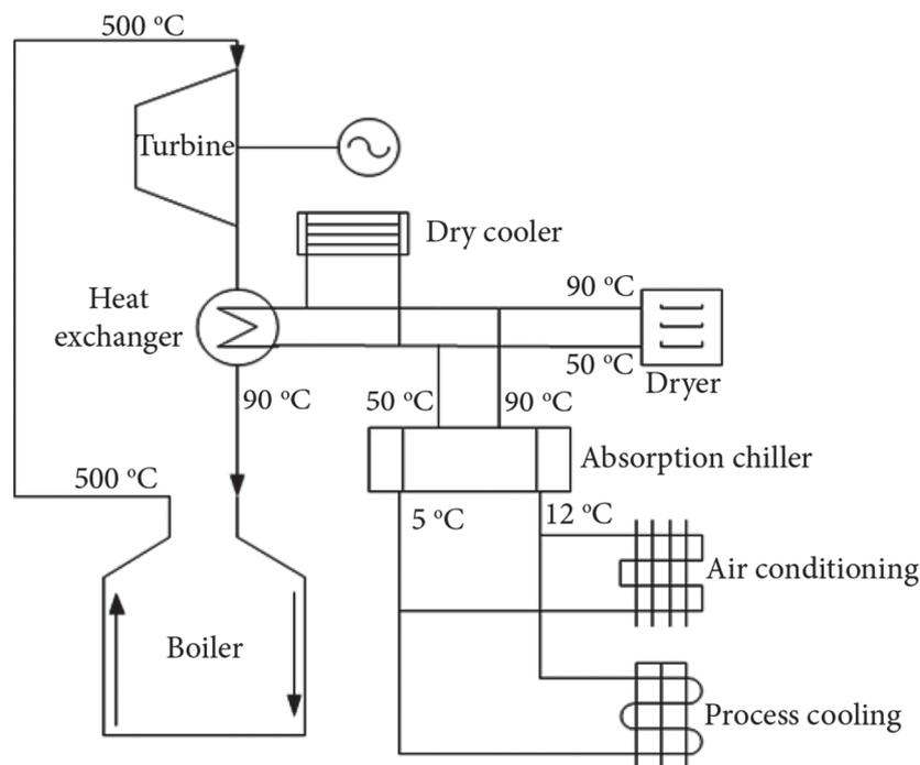
Fig. 3.7. Offered technological solution for the industrial CPs’ cooling system.
