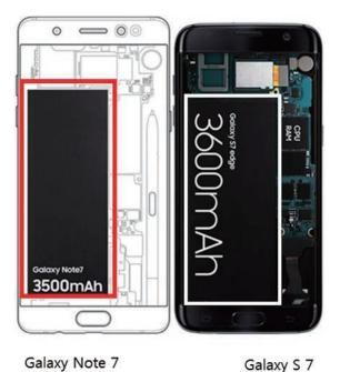
Fig. 3 Comparison between batteries of Galaxy Note 7 and Galaxy S7
