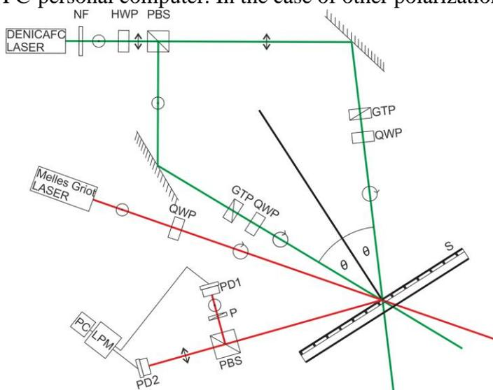
**Fig.3.** Experimental setup for reflection mode PA measurements. Notations are explained in the text.
