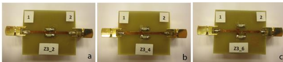
2.88. att. Spiestās plates z3. a – d = 2 mm, b – d = 4 mm, c – d = 6 mm.
