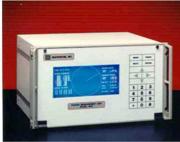
Figure 2.4 Macrodyne Inc. Developed PMU “Model 1690” ([www.macrodyneusa.com](http://www.macrodyneusa.com))
