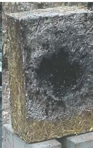
Fig. 5. Outer look of the slab after exposure to open fire.
