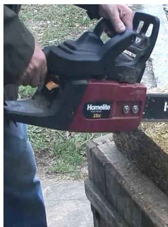
Fig. 2. Sawing of a straw-boon slab with a chain saw in transverse direction.
