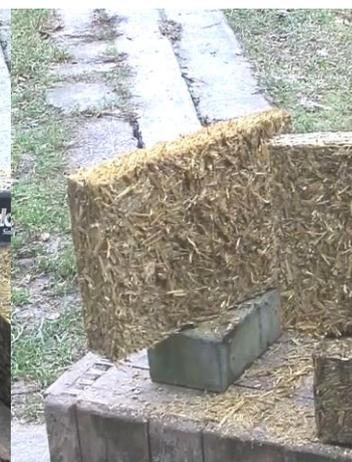
Fig. 3. Absence of angle and rib chips, smooth surface along the transverse sawing line.
