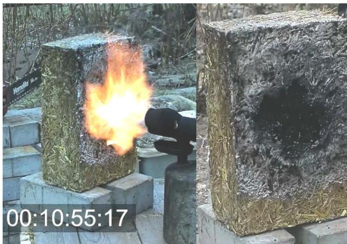
Fig. 4. Impact of fire on the slab during the test.
