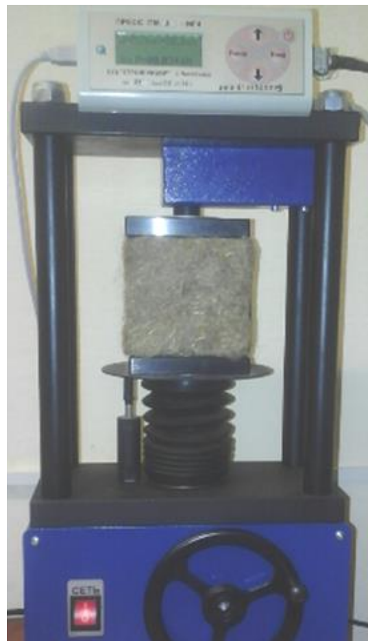
Fig. 2. Compressive strength test at 10 % deformation on ИМ-2МГ4 press.
