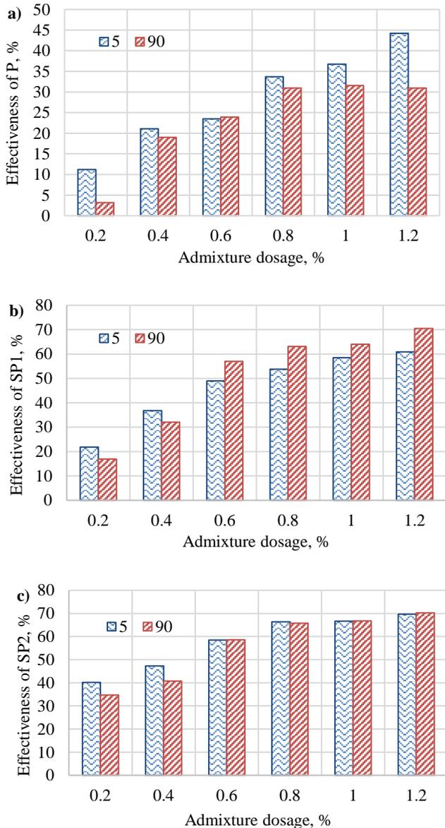
Fig. 14. The changes of effectiveness of (a) plasticizer P, (b) superplasticizer SP1 and (c) superplasticizer SP2 in cement pastes 5 and 90 min after mixing of the pastes.
