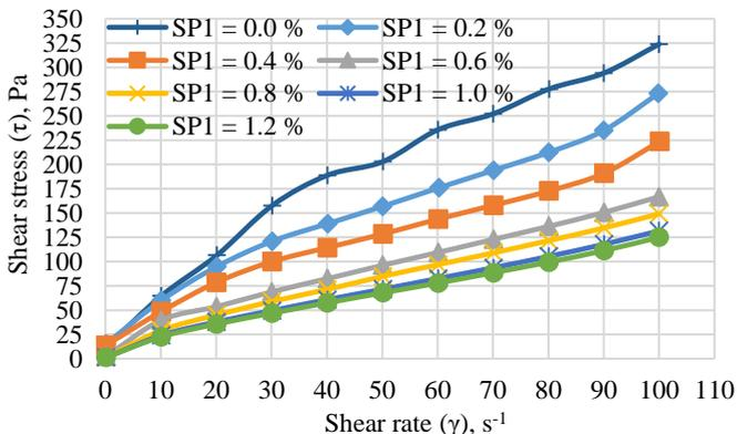
Fig. 6. Flow curves of cement pastes with superplasticizer SP1 5 min after mixing of the pastes.
