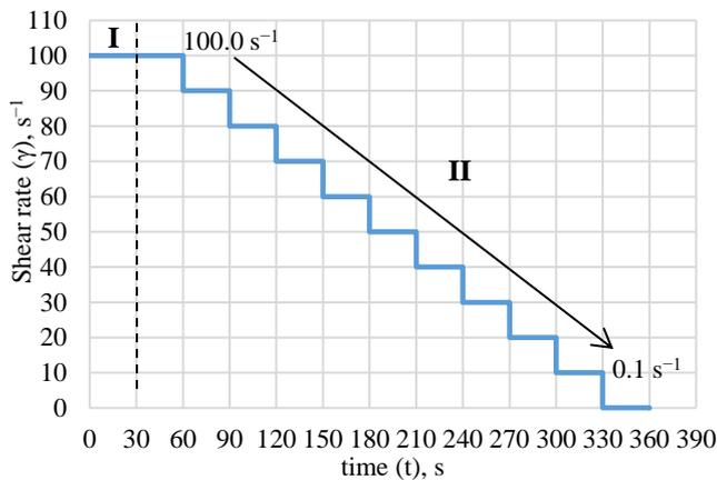
Fig. 3. Shear rates during testing vs. testing time.
