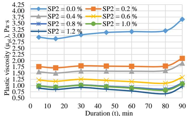
Fig. 13. Change of plastic viscosity of plasticized cement pastes with superplasticizer SP2 within 90 min duration.
