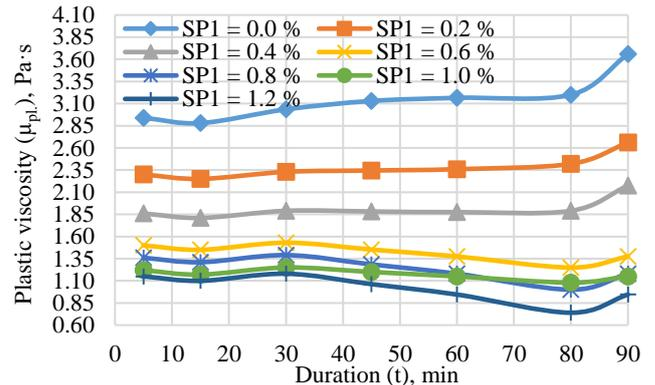
Fig. 12. Change of plastic viscosity of plasticized cement pastes with superplasticizer SP1 within 90 min duration.
