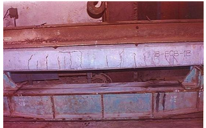
Fig. 8: Crack patterns in beam B-E-1B (beam with transverse reinforcement).
