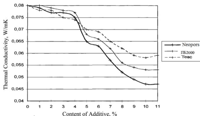
Fig. 4. Influence of the type and content of foam-forming additives on the thermal conduction of peat-wood insulation material.
