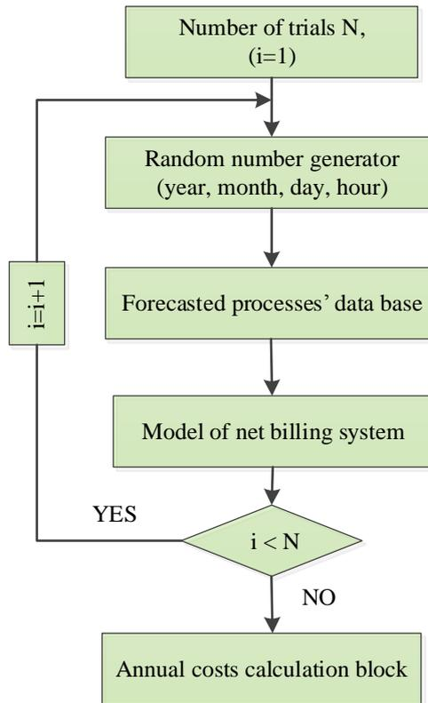
Fig. 3.2. The algorithm structure.
