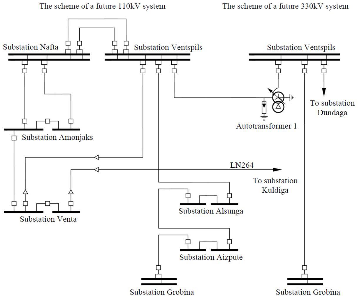
Fig. 4.1. Layout of a future cooperative circuit consisting of 110 kV and 330 kV systems.
