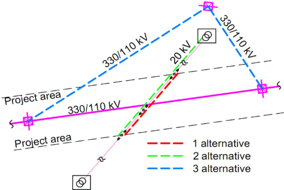
Fig. 4.2. Layout of PTL reconstruction design with solution alternatives.
