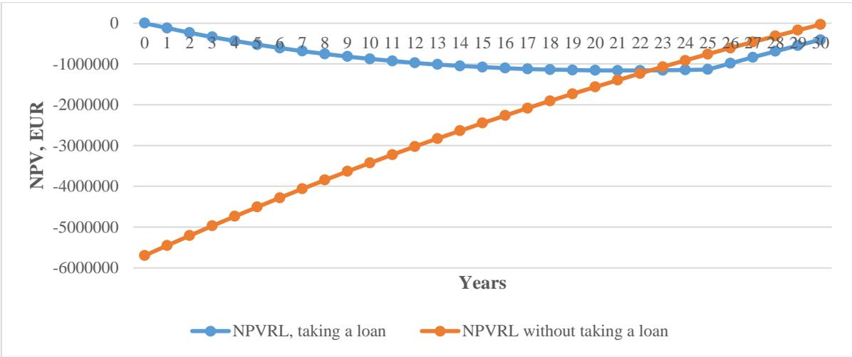
Fig. 3.6. NPV<sub>RL</sub> for the NET case (including the connection investments).
