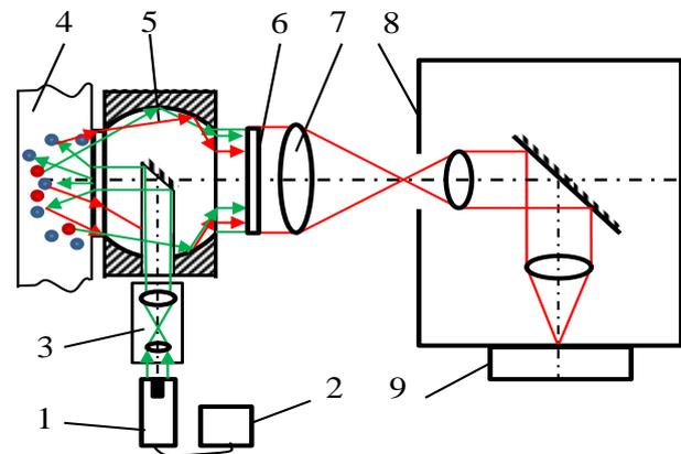
Fig.1. Structural and fundamental scheme of the setup for *in vivo* Raman spectroscopy by ellipsoidal reflectors: green colour – incident light; red colour – Raman scattering; 1 – laser light source; 2 – power regulator; 3 – optical collimator; 4 – biological object; 5 – optical block with ER; 6 – filter; 7 – lens; 8 – spectrograph; 9 – CCD camera.
