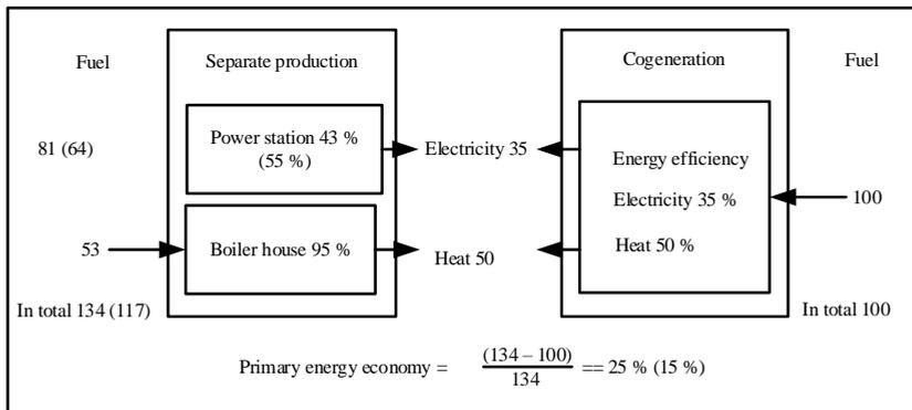
Fig. 10. Comparison of cogeneration and separate energy production.
