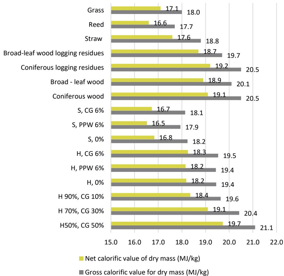
Fig. 2.19. A comparison of calorific values between existing solid biomass fuels and tested samples.
