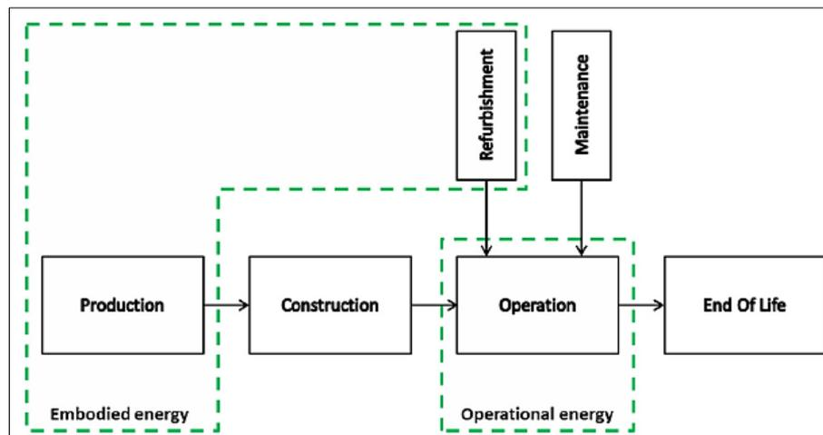
Figure 3.3: Embodied and operational energy interrelation in building's life cycle. [16]
