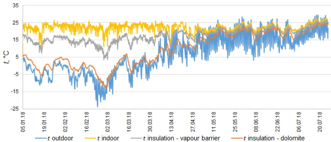
Fig. 2.14. Case building 2. Measured temperature at the interfaces of the living room wall.
