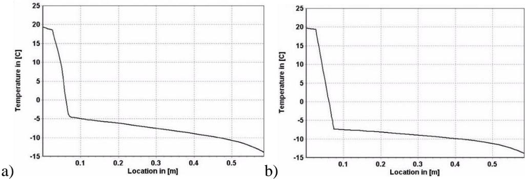
Fig. 2.20. Case building 1. Simulated temperature distribution (23 January at 9 a.m.) in the wall insulated with a) aerogel; b) VIP (outdoor on the right and indoor on the left of both graphs).
