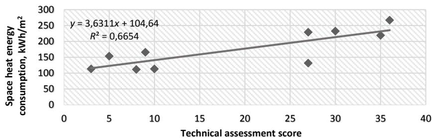
Fig. 2.1. Consumption of space heating energy related to building's technical assessment.
