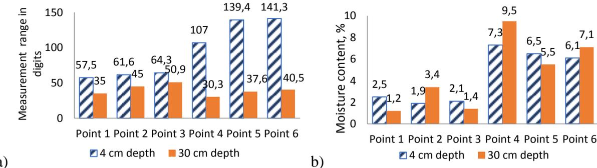
Fig. 2.3. Moisture measurements in Case building 1: a) non-destructive measurements with Trotec T600 and Trotec T650; b) destructive moisture content measurements.
