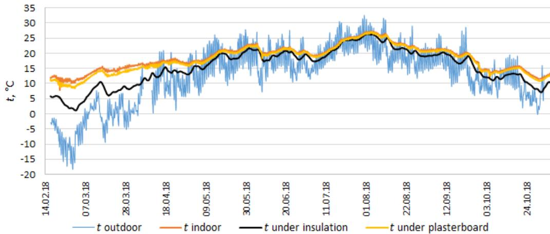
Fig. 2.17. Case building 3. Temperature measurements of the wall on the 1st floor.
