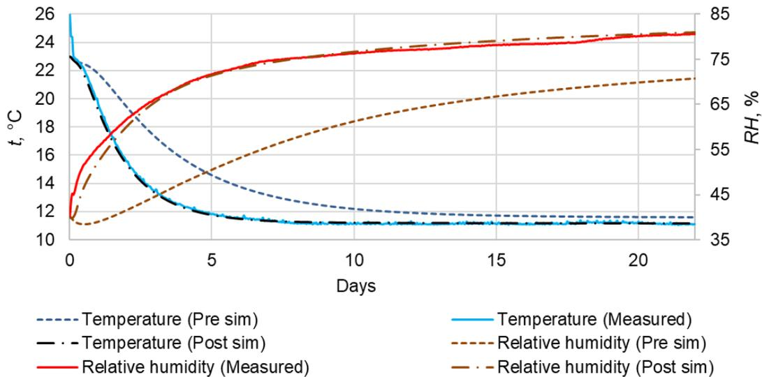
Fig. 2.9. Behaviour of temperature and relative humidity between masonry and wood fibre without vapour barrier insulation layer: simulation before and after the experiment, and measured results.
