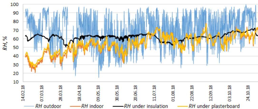
Fig. 2.18. Case building 3. Relative humidity measurements of the wall on the 1st floor.
