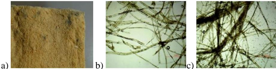
Fig. 2.7. Mould on wood fibre mat after the test: a) mould on the top right corner; b) magnified wood fibre without mould; c) with mould.
