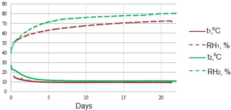
Fig. 2.6. Measured temperature and relative humidity between masonry and wood fibre:  $t_1$ ,  $RH_1$  – without vapour barrier;  $t_2$ ,  $RH_2$  – with vapour barrier.
