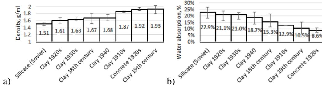
Fig. 2.4. Laboratory test results: a) dry density; b) water absorption.
