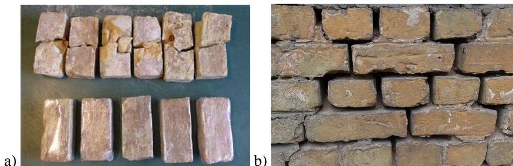
Fig. 2.5. a) Bricks after 15 frost-thaw test cycles: fully saturated samples (~36 %) in upper row, while samples saturated to 20 % in bottom row; b) extensive loss of mortar due to high presence of sulphates.
