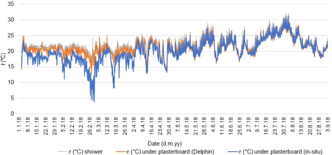
Fig. 2.23. Case building 2. Temperature of the bathroom wall between insulation and vapour barrier.
