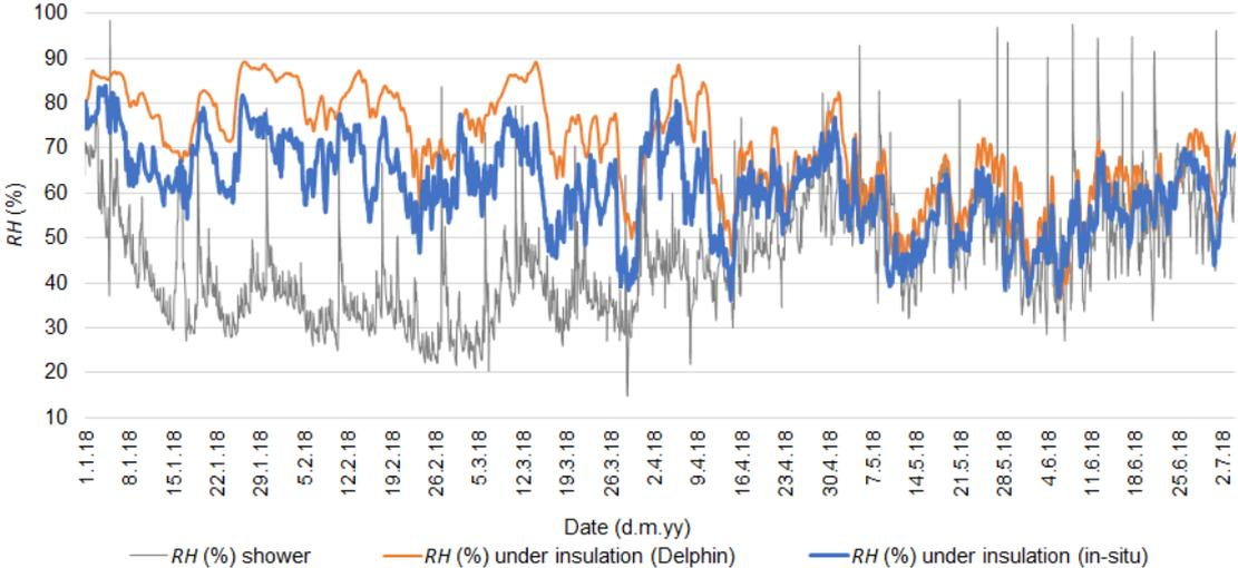
Fig. 2.24. Case building 2. Relative humidity of the bathroom wall between dolomite and insulation layers.
