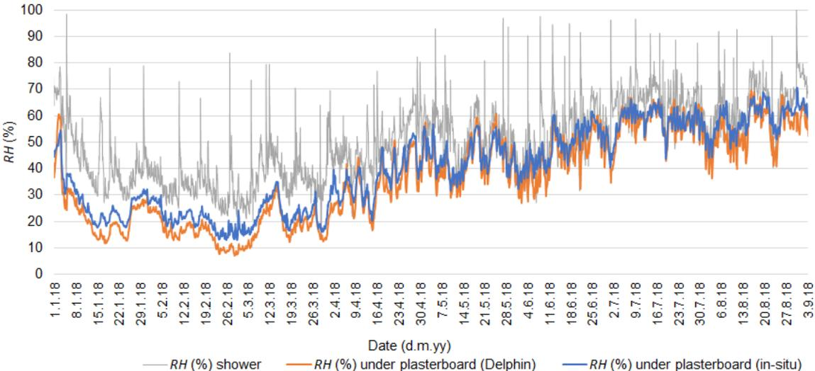
Fig. 2.22. Case building 2. Relative humidity of the bathroom wall between insulation and vapour barrier.
