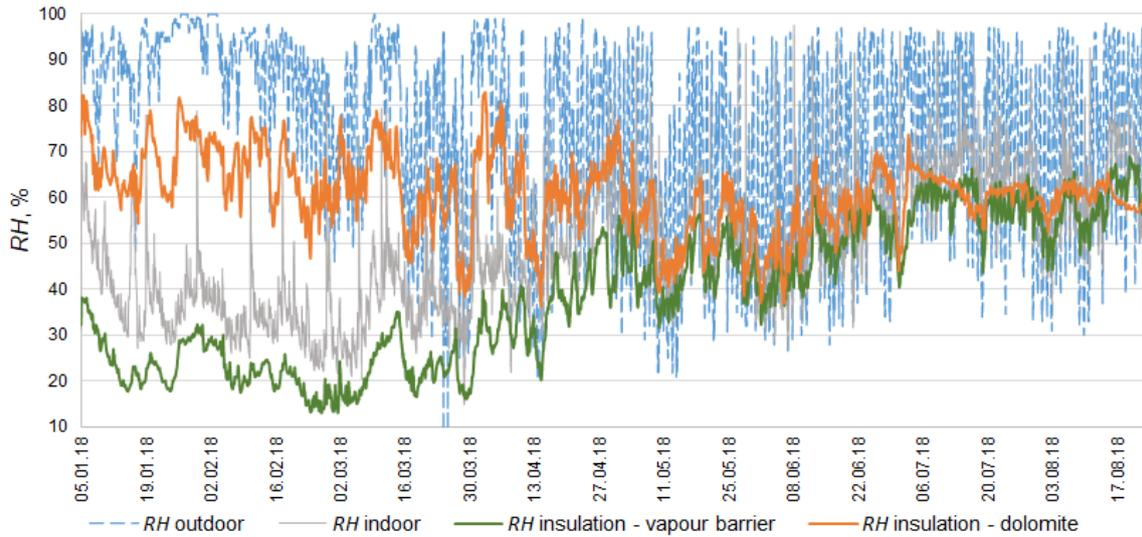
Fig. 2.15. Case building 2. Measured relative humidity at the interfaces of the bathroom wall.
