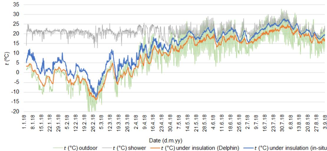
Fig. 2.25. Case building 2. The temperature of the bathroom wall between dolomite and insulation layers.
