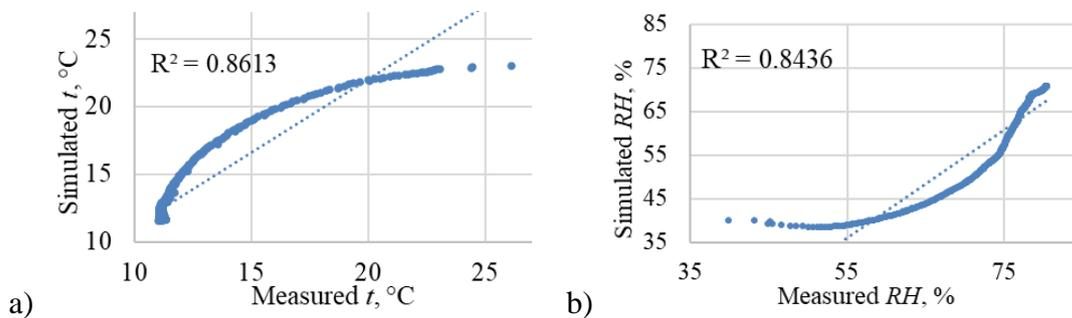
Fig. 2.8. Correlation between simulated and measured data for wood fibre:
