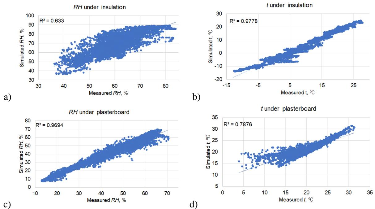
Fig. 2.26. Correlation between simulated and measured data in the bathroom wall: a) relative humidity between dolomite and insulation; b) temperature between dolomite and insulation; c) relative humidity between insulation and plasterboard; d) temperature between insulation and plasterboard.
