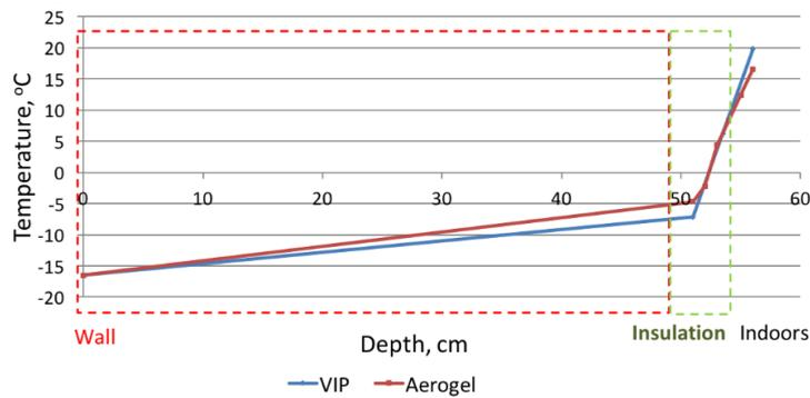
Fig. 2.12. Measured temperature distribution in the wall construction at the lowest outside temperature (−16.5 °C).
