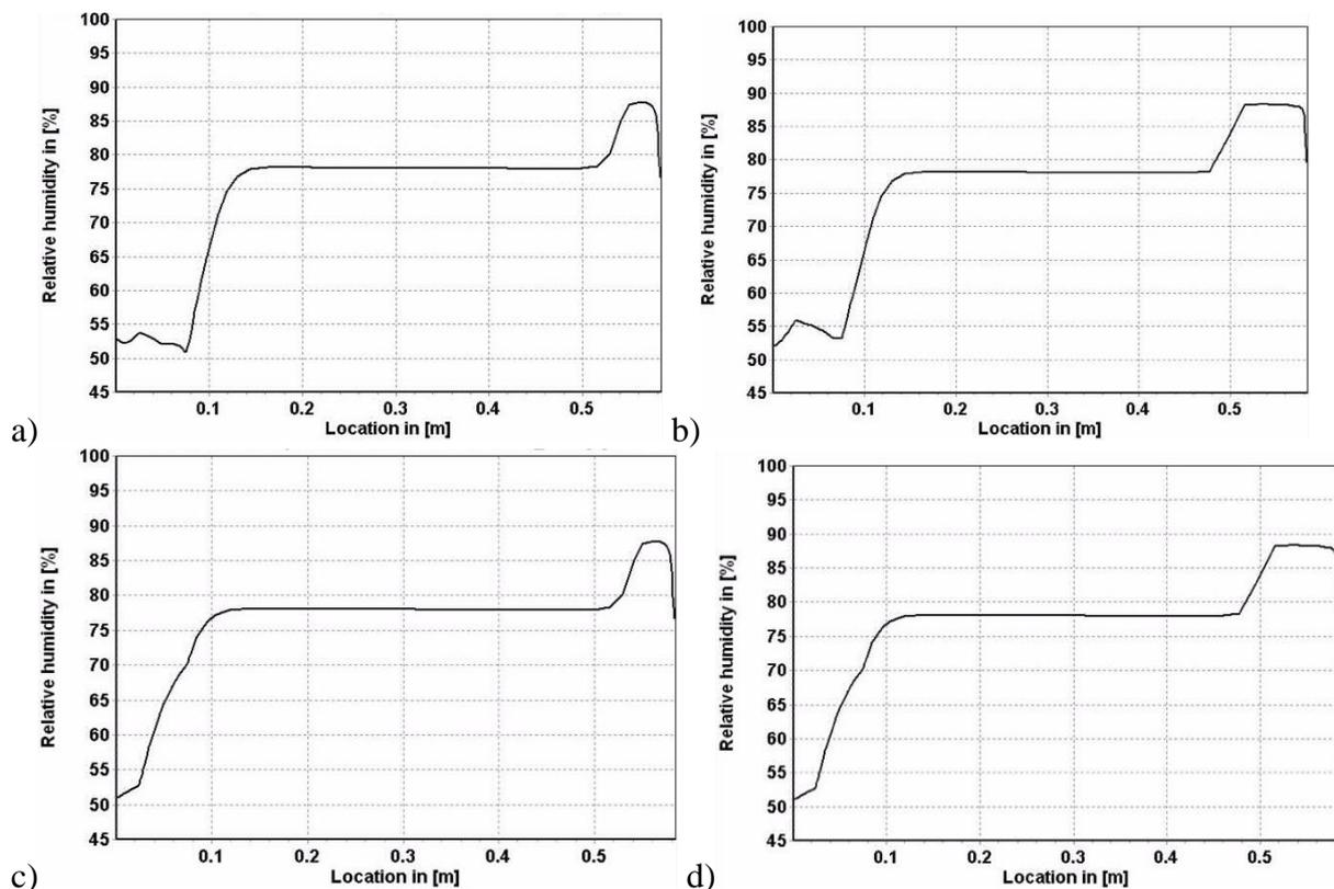
Fig. 2.21. Case building 1. Simulated *RH* in the wall (23 January at 9 a.m.) insulated with: a) aerogel and water repellent hydrophobic paint; b) aerogel and without paint; c) VIP and water repellent hydrophobic paint; d) VIP and without paint; (outdoor on the right and indoor on the left of both graphs).
