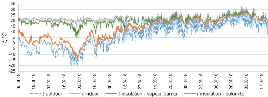
Fig. 2.16. Case building 2. Measured temperature at the interfaces of the bathroom wall.
