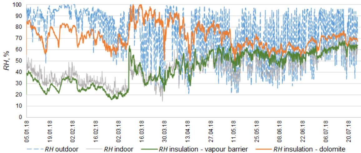
Fig. 2.13. Case building 2. Measured relative humidity at the interfaces of the living room wall.
