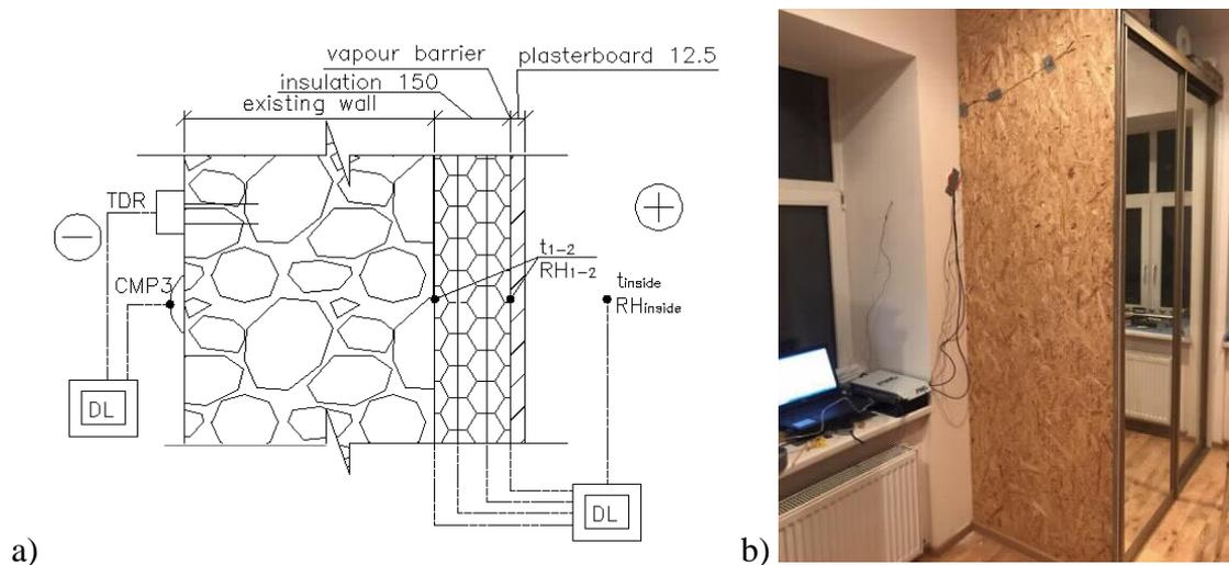
Fig. 1.2. a) Measurement setup for Case building 2 ( $t$  – temperature;  $RH$  – relative humidity;  $CMP3$  – sun radiation,  $DL$  – data logger,  $TDR$  – volumetric water content.);
