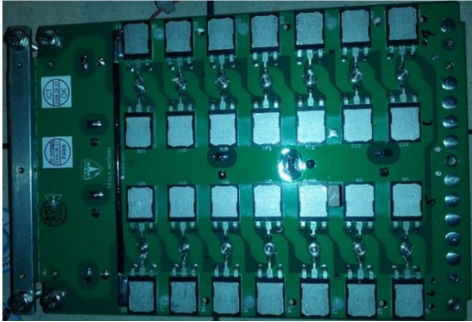
Figure 3.8: TESLA Model S half-bridge inverter power PCB.
