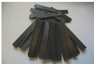
Fig. 1. WPC samples for water uptake study
