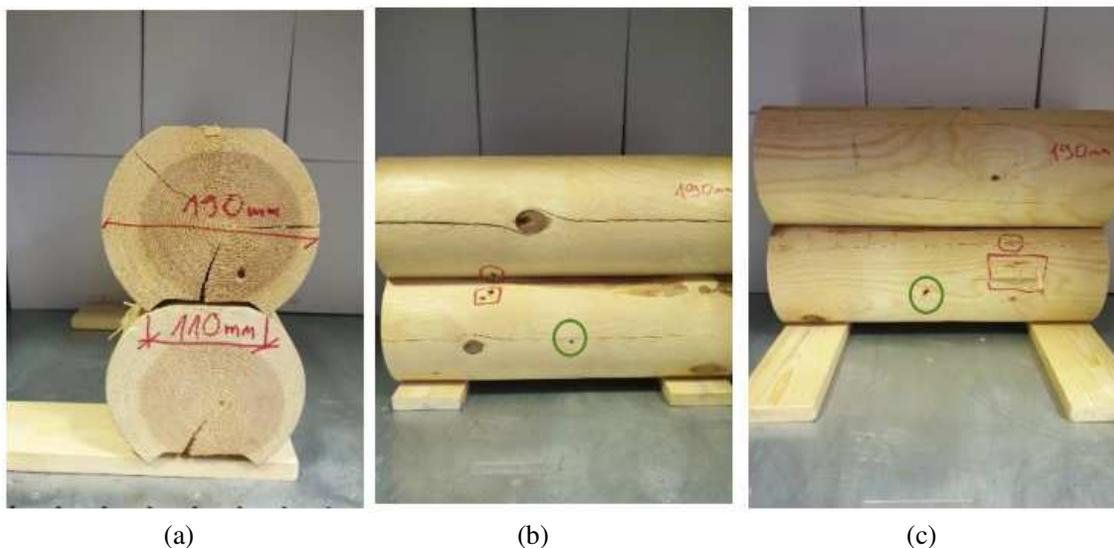
**Figure 1.** (a) Dry pine log samples after shooting - side view; dimensions in red. Log width 190 mm, narrowest joint 110 mm; (b) (c) Samples of pine log after firing (b) bullet entry side (c) bullet output side; the red mark indicates the location of the three bullets fired by the Glock 17, and the green mark indicates the bullets fired by the larger APC556.
