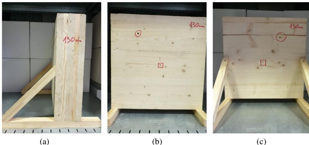
**Figure 3.** 130 cm (30-20-30-20-30 mm) thick CLT target; (a) side view; tripod shown; (b) bullet input; (c) bullet output.
