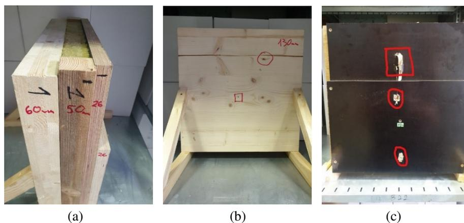
**Figure 5.** Combined panel (a) side view; (b) bullet entrance; (c) bullet output.
