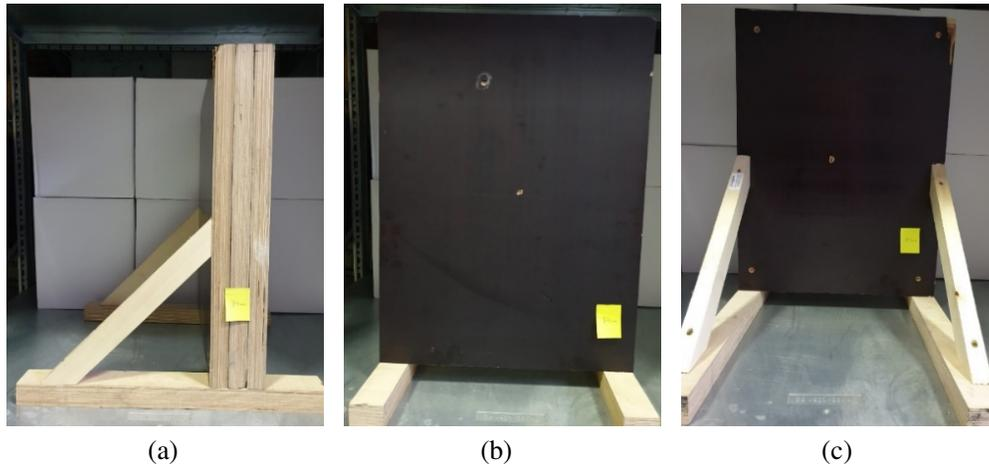
**Figure 2.** 84 cm plywood target - 3 plates assembled; (a) side view; tripod shown; (b) bullet input; (c) bullet output side.
