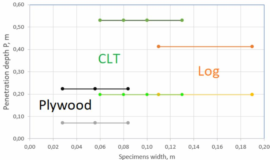
**Figure 4.** Penetration depth  $P$  for each group of specimens.
