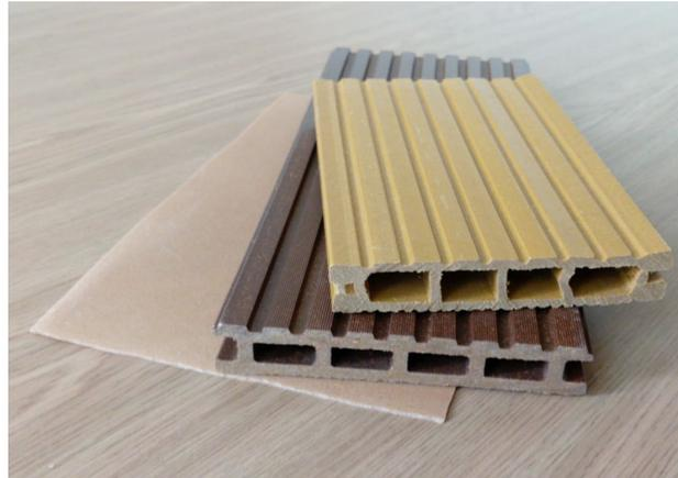
Figure 3.12. Melt compounded wood polymer composites decks and sheets profiles.
