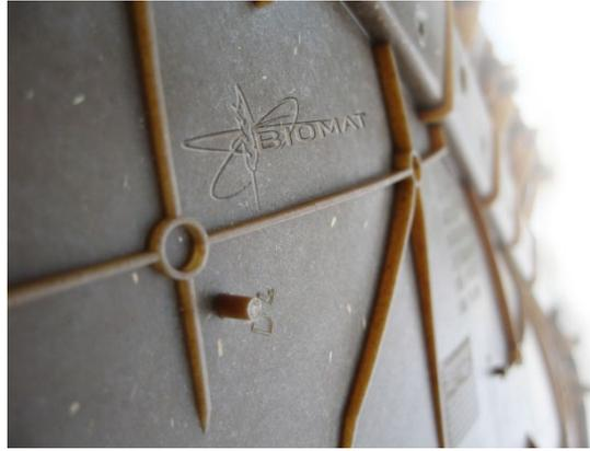
Figure 1.13. Injection molded PBS/hemp custom interior panel [209].
