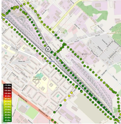
Fig. 3.12. Tele2 2G MCN radio coverage measurements at Skirotava station.
