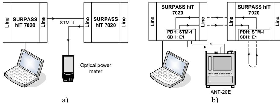
Fig. 3.15. Connection schemes: a) for optical power measurement; b) for PDH/SDH analysis.
