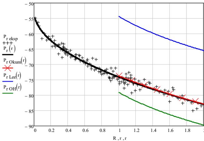
Fig. 3.13. Experimentally obtained MS power curve  $P_r(r)$ , compared with mathematical models of radio wave propagation (Okumura, Lee, Okumura-Hata).
