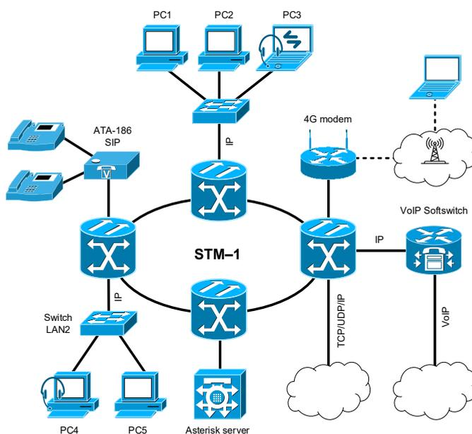
Fig. 3.14. Heterogeneous network diagram.
