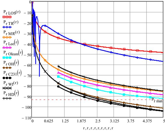
Fig. 3.9. Comparison of the radio signal power at the reception point  $P_r$  (dBm) as a function of the distance between the BTS and the MS (in downlink mode) for the mathematical models.
