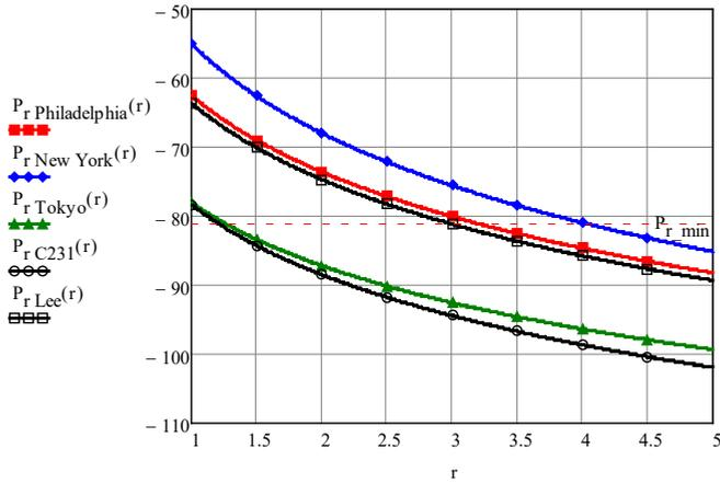
Fig. 3.10. Theoretical and experimental values of MS received signal power.
