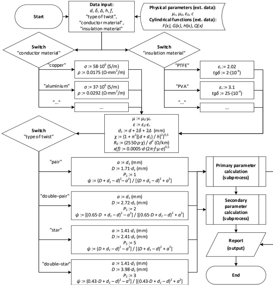
Fig. 3.4. The algorithm for calculating the parameters of SCCL in Mathcad.
