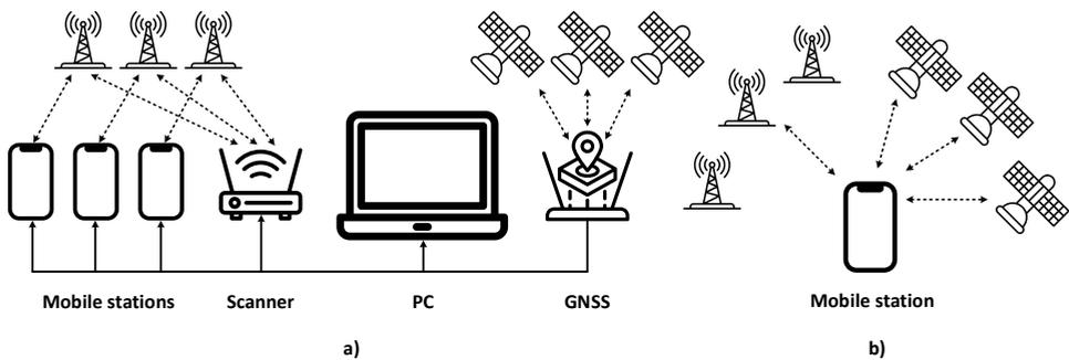
Fig. 3.11. MCN parameter measurement methods: a) active; b) passive.
