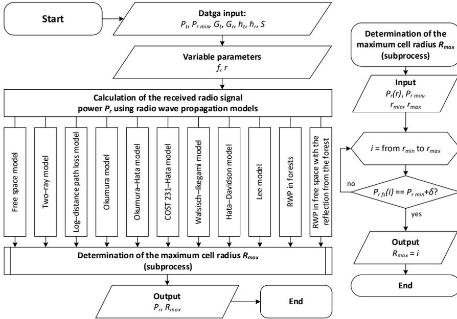
Fig. 3.8. Algorithm for calculating the maximum radius of an MCN cell.
