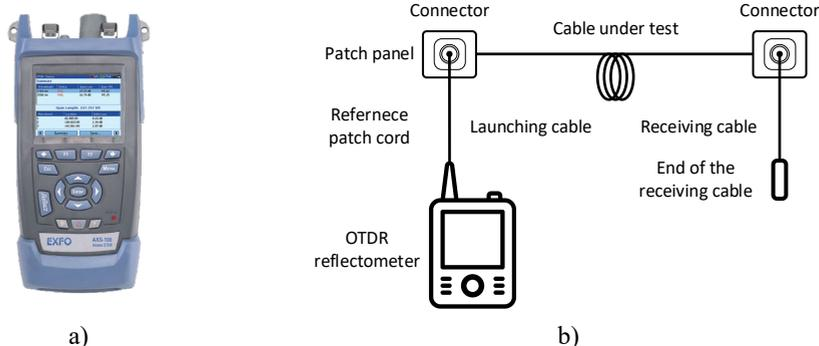
Fig. 3.7. EXFO AXS-100 OTDR reflectometer external appearance (a) and connection diagram (b).
