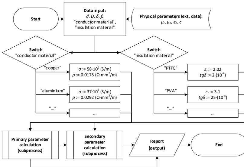
Fig. 3.5. Algorithm for calculating the CCCL parameters in Mathcad.
