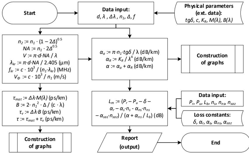
Fig. 3.6. Algorithm for calculating the parameters of the FOCL in Mathcad.
