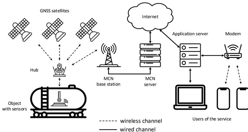
Fig. 3.1. Example of a telematics system and its equipment.
