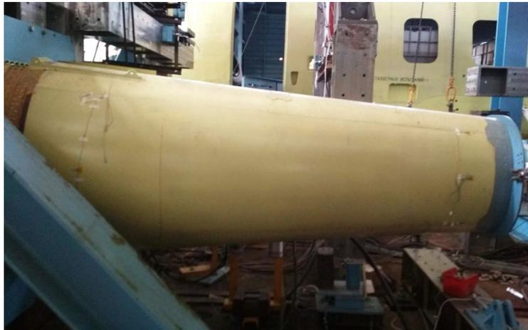
Fig. 5.3. The tail beam of the Ka-62 helicopter on the test bench.
