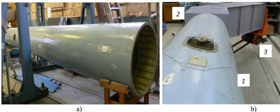
Fig. 5.1. General view of the helicopter Mi-8 tail beam (a) and the test setup for dynamic loading (b); 1– the tail beam, 2 – imitator of the tail rotor beam, 3 – the eccentric shaker.
