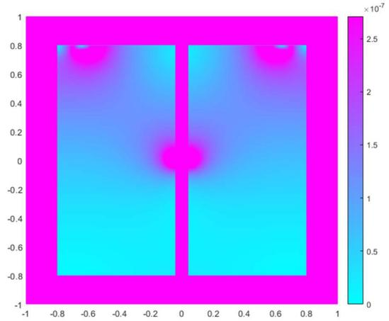
Fig. 4. Magnetic flux density when rotor and stator tooth are in front of each other ( $\alpha^E=0$ ) and  $\mu_{iron} = 4 \cdot 10^4$
