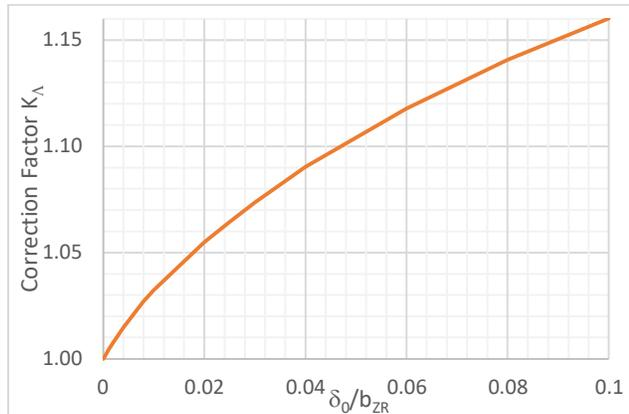
Fig. 10. Correction factor  $K_\Lambda$  for the maximum permeance calculation
