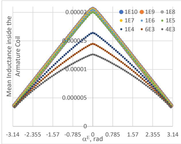
Fig. 6. Mean magnetic inductance vs rotor rotation angle of elementary tooth section of a HIA with various iron magnetic permeability and typical rotor slot depth
