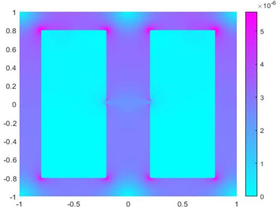
Fig. 8. Magnetic field pattern in the air gap when  $\delta_0/b_{ZR} = 0.1$
