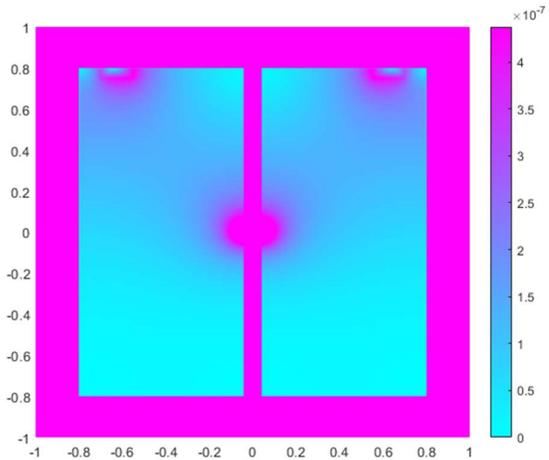
Fig. 5. Magnetic flux density when rotor and stator tooth are in front of each other ( $\alpha^E=0$ ) and  $\mu_{iron} = 1 \cdot 10^{10}$
