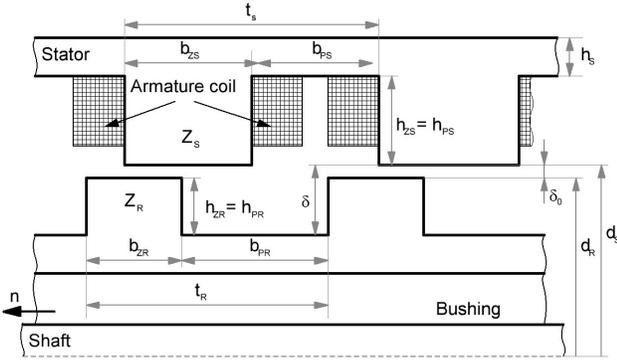
Fig. 1. Sweep of the teeth zone of a HIA with concentrated-type armature winding (one pack is shown)
