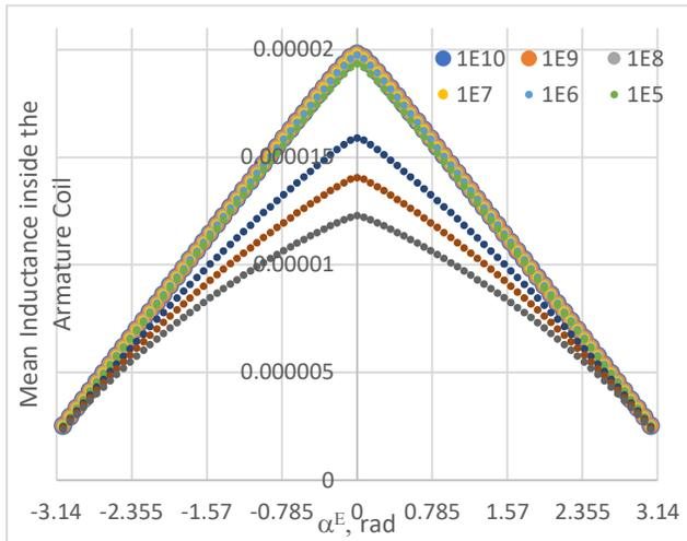
Fig. 3. Mean magnetic inductance vs rotor rotation angle of elementary tooth section of a HIA with various iron magnetic permeability and "deep" rotor slot
