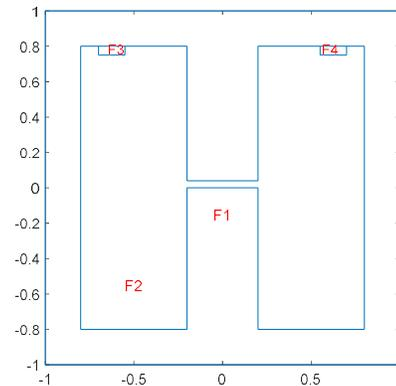
Fig. 2. Structure of the Magnetic Circuit: F1 – iron, F2 – air, F3,F4 – field coils
