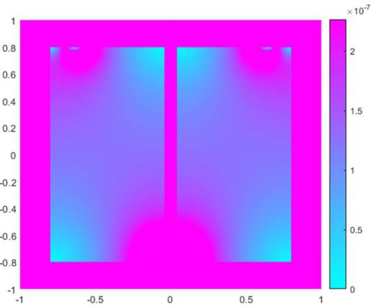
Fig. 7. Magnetic flux density when rotor and stator tooth are in front of each other ( $\alpha^E=0$ ) and  $\mu_{iron}=1 \cdot 10^{10}$  for a typical rotor slot depth
