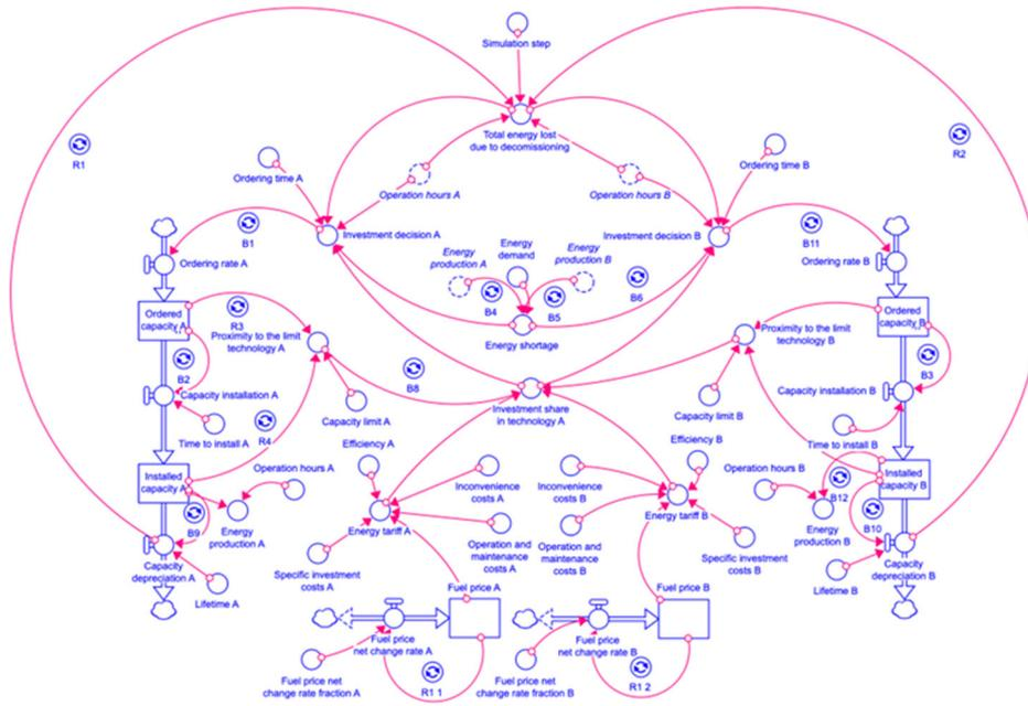
Fig. 1.2. Structure of stocks and flows in the energy supply sector.
