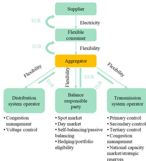
Fig.1.4. Flexibility services provided by the aggregator
