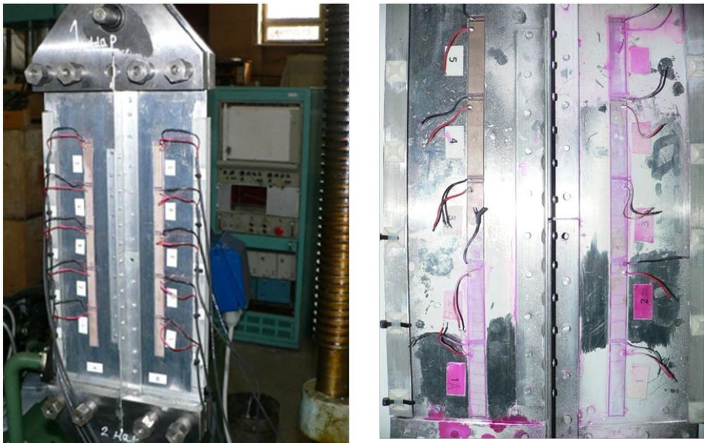
Fig. 2.1. A forced panel prepared for fatigue test and installed in machine GRM-20 (to the left) and the view of the panel after the penetration test (to the right) for finding the crack in PZT transducers.
