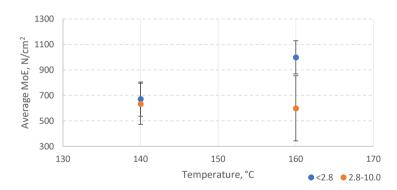
Fig. 2.5. Modulus of elasticity of  $\leq$  2.8 mm particle size boards (blue), and for 2.8–10.0 particle size boards (orange) depending on the hot press temperature for combined particles.
