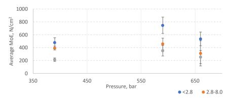
Fig. 2.3. Modulus of elasticity depending on pressure and particle size: < 2.8 mm particle size boards; 2.8–8.0 mm particle size boards; 10.0 mm particle size boards. MoE – modulus of elasticity
