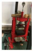
Fig. 1.1. Hydraulic hot press.
