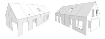
Fig. 1.5. 3D representation of the individual house CLT weight bearing construction.
