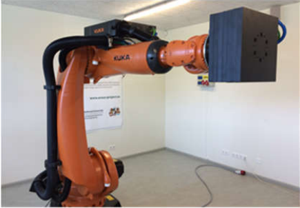
Fig. 4. Industrial robot manipulator equipped for toll mass variation related experiment.
