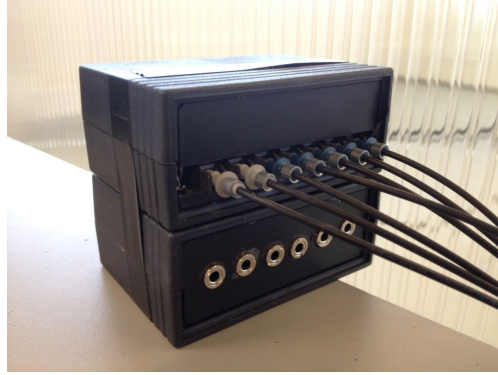
Fig. 3.21. Optical fiber data transmission and aggregation device.
