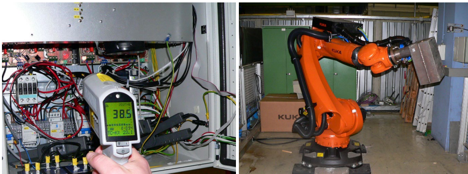
Fig. 2.7. Experimental verification in production area: interconnection module with peripheral devices (left) and one of the interconnected KUKA KR210 industrial robots (right).
