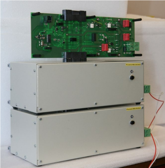
Fig. 2.15. A practically implemented modular solution for the DC link interconnection of industrial robots.
