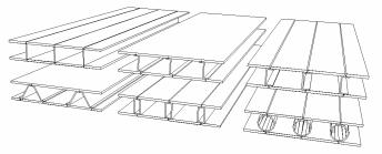
Figure 5. Schemes of metal sandwich panels of various core types
