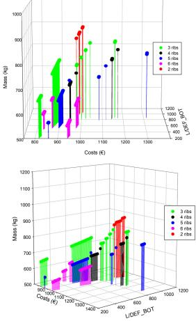
Figure 8. Pareto points for I core sandwich panel
