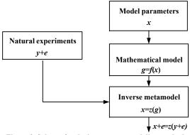
Figure 3. Scheme for the inverse metamodeling method
