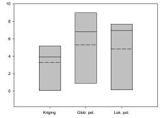
Figure 7. Approximation error for various responses for the I core panel in 250 test points, using kriging, polynomial and locally weighted polynomial approximations
