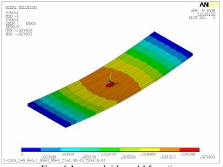
Figure 6. I core sandwich panel deformation
