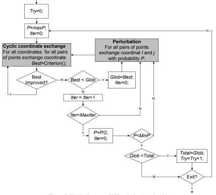
Figure 2. Block diagram of LH optimization algorithm
