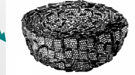
Fig.2 Illustrative example of extremely high structure carbon black particle [W.Hofman, H.Gupta, Kautchuk technology, Doktor Gupta Verlag, 2001, p.16]
