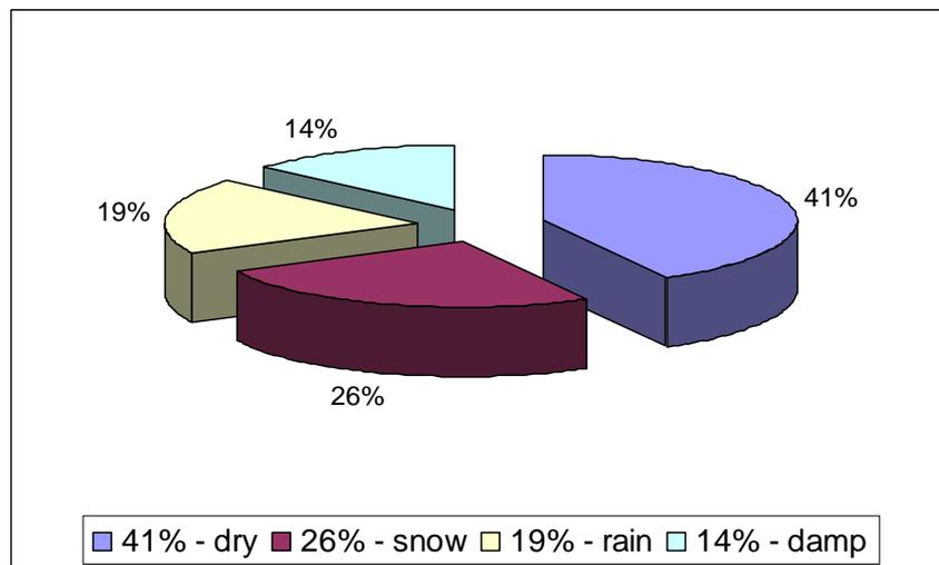
Fig. 1.3. Connection between wagon derailment and weather conditions
