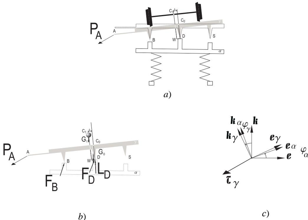
Fig. 2.3. Analytical model for defining balance conditions of laboratory assembly, loaded with probing effect of force  $P_A$ ;
