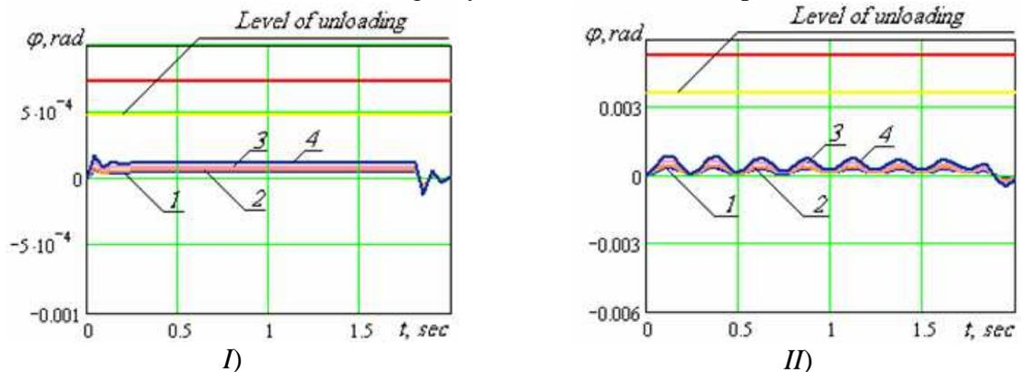
Fig. 4.3. Amplitudes of angle  $\varphi$  changes for the first wagon of cut, consisting of 3 covered wagons, approaching retarding interval at the speed of  $v_0$ , appearing as a result of braking:
