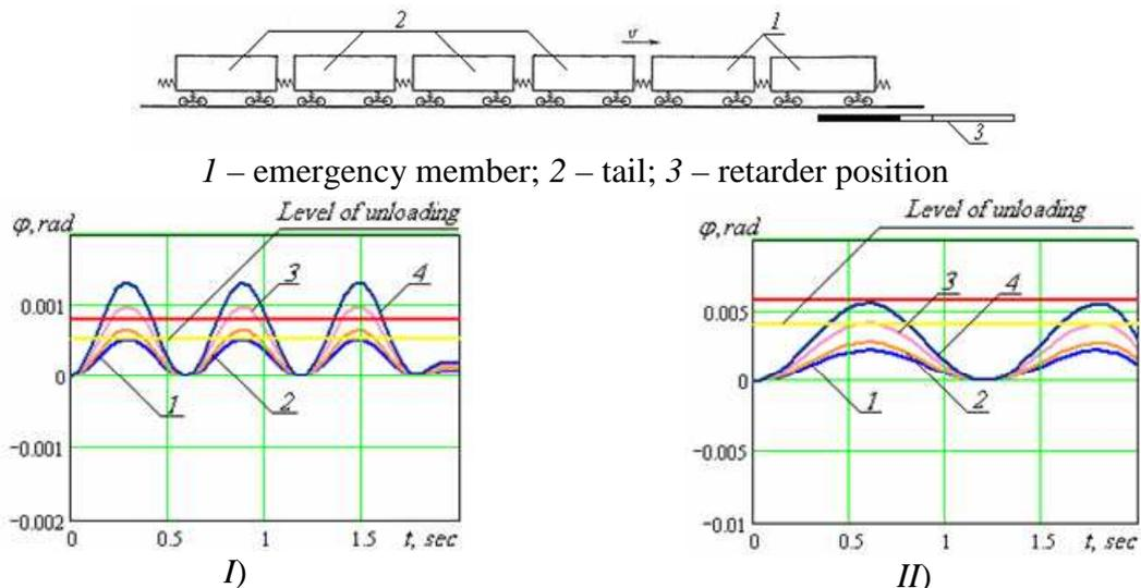
Fig. 4.7. Amplitudes of angle  $\varphi$  changes for the third wagon of cut, consisting of 6 open wagon, approaching retarding interval at the speed of  $v_0$ , appearing as a result of braking:
