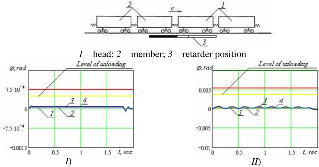
Fig. 4.6. Amplitudes of angle  $\varphi$  changes for the third wagon of cut, consisting of 4 platform, approaching retarding interval at the speed of  $v_0$ , appearing as a result of braking:
