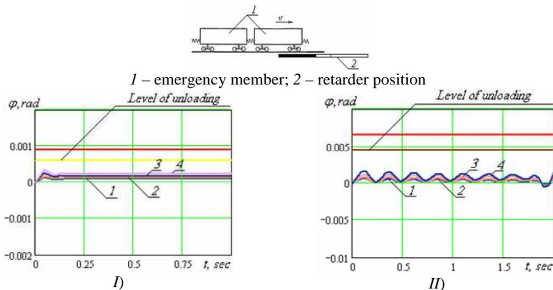
Fig. 4.1. Amplitudes of angle  $\varphi$  changes for the first wagon of cut, consisting of 2 *tank-wagons*, approaching retarding interval at the speed of  $v_0$ , appearing as a result of braking:
