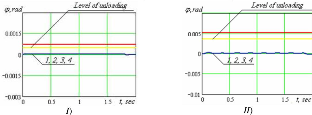
Fig. 4.12. Amplitudes of angle  $\varphi$  changes for the ninth wagon of cut, consisting of 10 *hoper cut*, approaching retarding interval at the speed of  $v_0$ , appearing as a result of braking:
