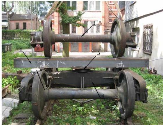
Fig. 2.1. Experimental assembly for defining moment by bogie rotation resisting force in supporting node:
