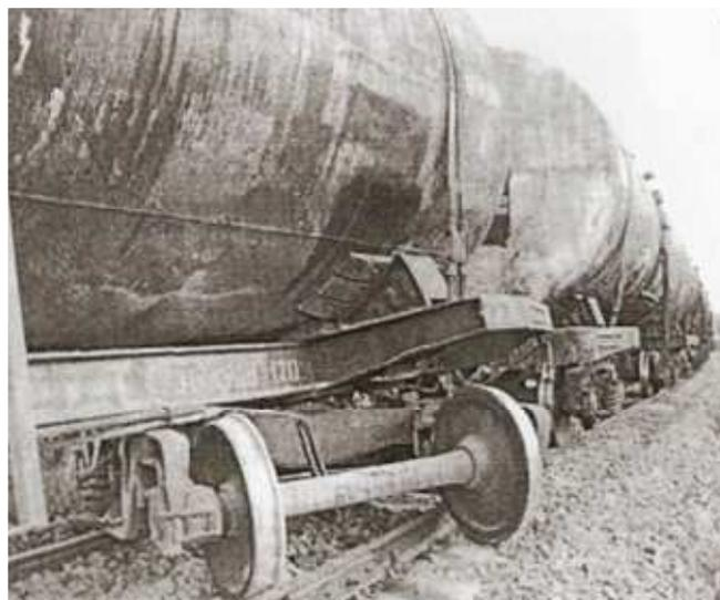
Fig. 1.5. Wagon derailment due to bogie jamming
