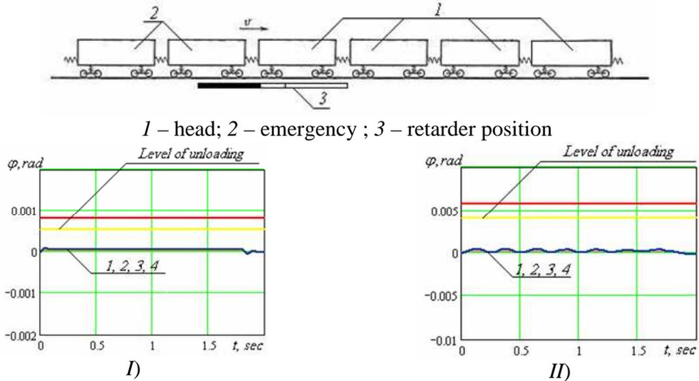
Fig. 4.9. Amplitudes of angle  $\varphi$  changes for the third wagon of cut, consisting of 6 *open wagon*, approaching retarding interval at the speed of  $v_0$ , appearing as a result of braking:
