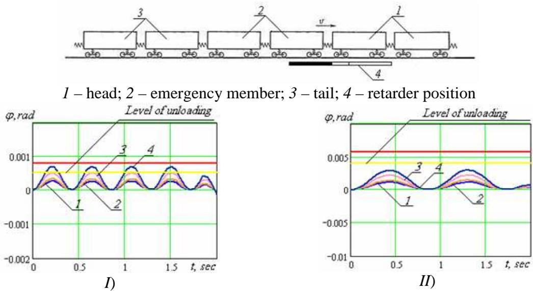
Fig. 4.8. Amplitudes of angle  $\varphi$  changes for the third wagon of cut, consisting of 6 *open wagon*, approaching retarding interval at the speed of  $v_0$ , appearing as a result of braking:
