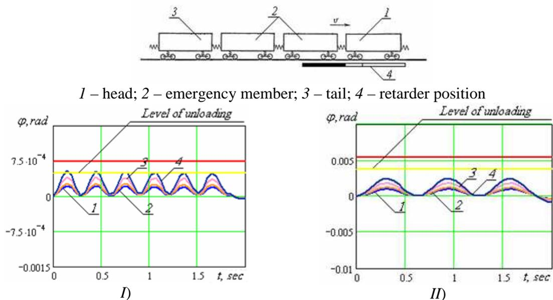
Fig. 4.5. Amplitudes of angle  $\varphi$  changes for the second wagon of cut, consisting of 4 platform, approaching retarding interval at the speed of  $v_0$ , appearing as a result of braking:
