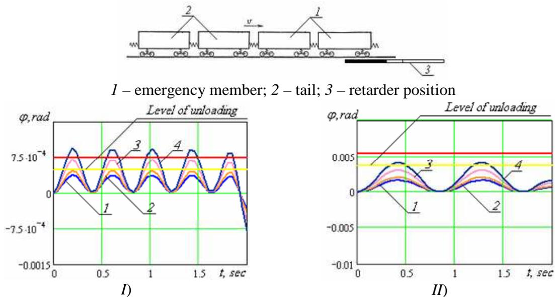
Fig. 4.4. Amplitudes of angle  $\varphi$  changes for the first wagon of cut, consisting of 4 platform, approaching retarding interval at the speed of  $v_0$ , appearing as a result of braking:
