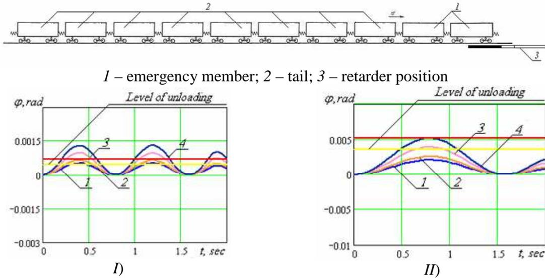
Fig. 4.10. Amplitudes of angle  $\varphi$  changes for the first wagon of cut, consisting of 10 *hoper cut*, approaching retarding interval at the speed of  $v_0$ , appearing as a result of braking:
