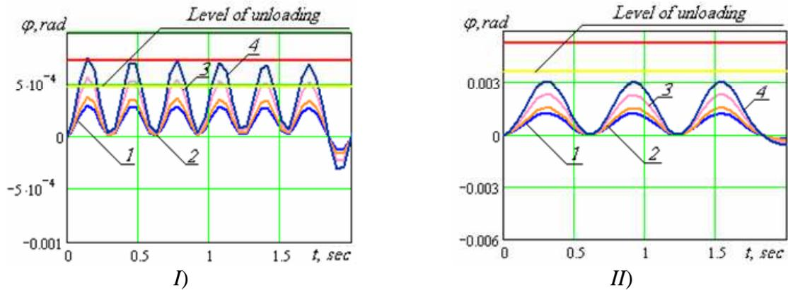
Fig. 4.2. Amplitudes of angle  $\varphi$  changes for the first wagon of cut, consisting of 3 covered wagons, approaching retarding interval at the speed of  $v_0$ , appearing as a result of braking:
