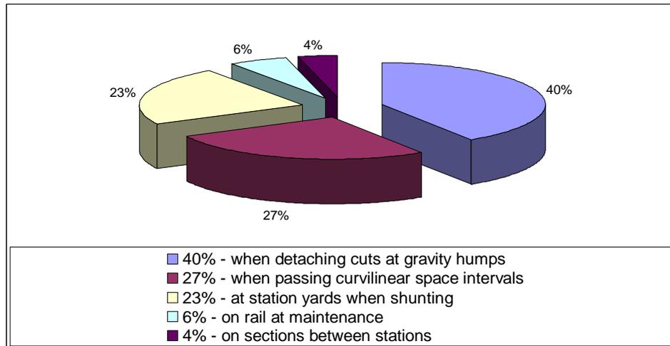
Fig. 1.4. Allotment of freight wagon derailment from 1997 to 2009
