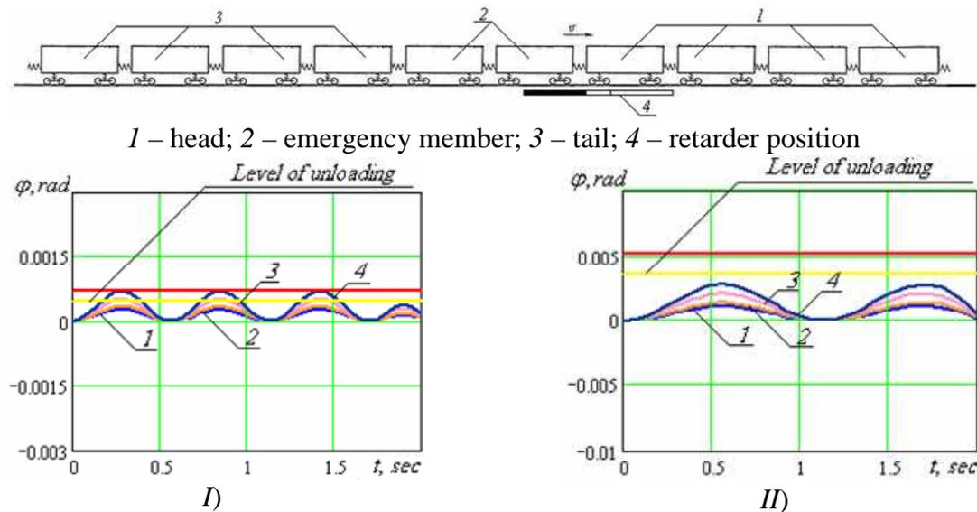
Fig. 4.11. Amplitudes of angle  $\varphi$  changes for the fifth wagon of cut, consisting of 10 *hoper cut*, approaching retarding interval at the speed of  $v_0$ , appearing as a result of braking:
