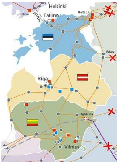
Fig. 7.1. Baltic 330 kV separated power transmission network
