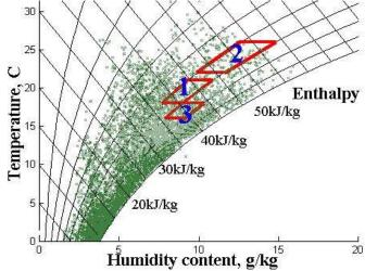
Fig.2.1. The air parameters of the outdoor air and the comfort areas of the animal house.
