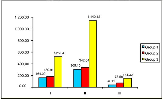
Fig.3.5. Annual consumption of energy of the  $1^{st}$ ,  $2^{nd}$  and  $3^{rd}$  ventilation systems for each group of pigs per 1 m<sup>2</sup> of the floor area in the piggery during the heating period.
