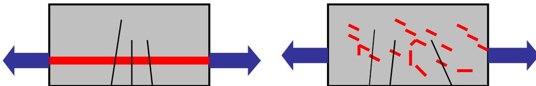
Figure 1. Long and short fibers reinforcement under tensile load in concrete (two different load bearing mechanisms)
