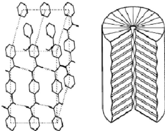
Figure 4. Aramid unit cell and fibre structure [5]
