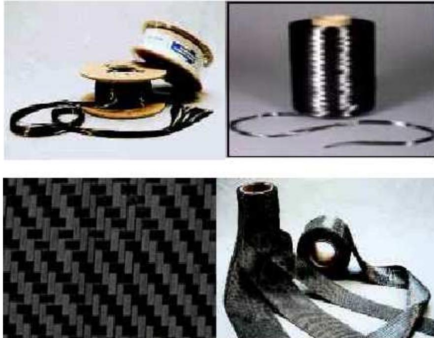
Figure 3. Samples of commercially available carbon fibre products (picture from [3])
