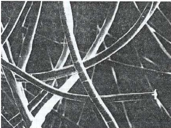
Figure 5. Extruded ordinary polypropylene fibers (picture from [7])
