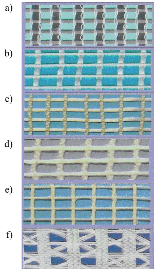
Figure 8. Fibre nets for concrete reinforcement (picture from [11])
